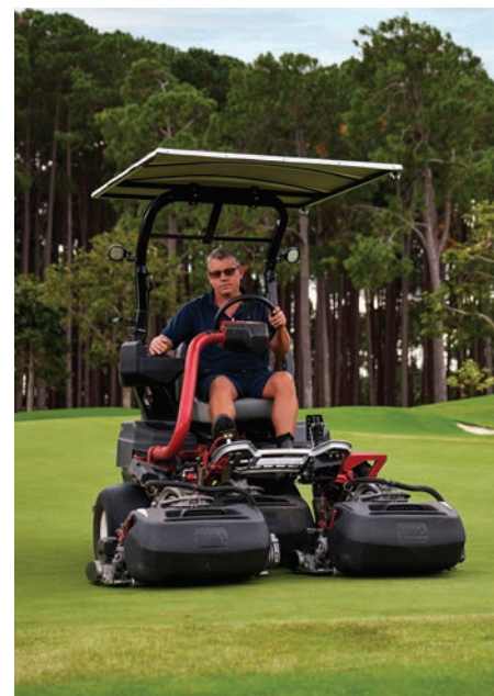
Powered by eight lithium-ion Samsung SDI batteries, the Greensmaster® eTriFlex™ 3370 carries no hydraulic fluid and utilises all-electric components for traction, steering, lifting and cutting
