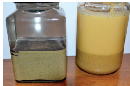
A simple jar test can be used for a quick visual inspection of a sand's characteristics
