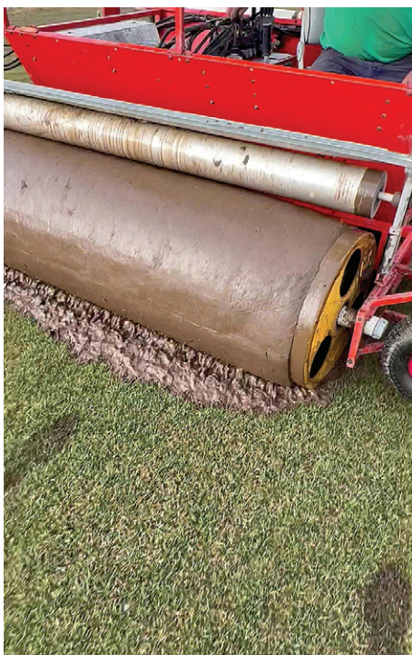
Following the early July 2022 inundation, silt was removed by flooding the turf with fresh water and using a Super Sopper to lift the silt which was then pushed off the pad
