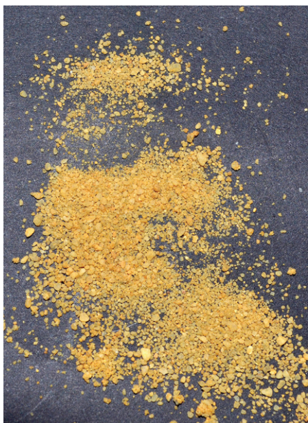
Knowledge of characteristics such as particle size distribution is critical when determining a sand for topdressing or construction purposes
