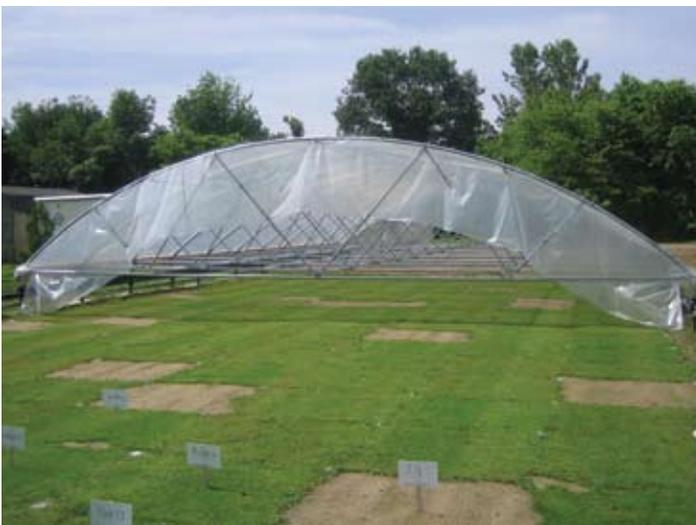
*UMASS Drought Resistant Turf Study. This cover will automatically cover the turf when it starts to rain.*
