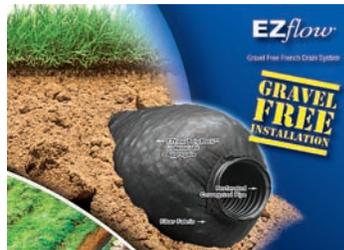
This product is a 10 foot long slotted pipe surrounded by Poly Rock and enclosed in a geotextile mesh.
