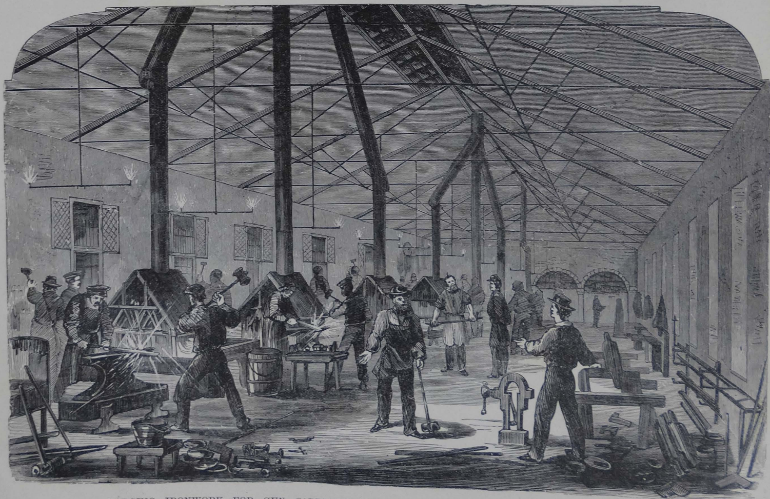
FORGING IRONWORK FOR GUN CARRIAGES AT THE WATERVLIET ARSENAL, WEST TROY, N. Y.
