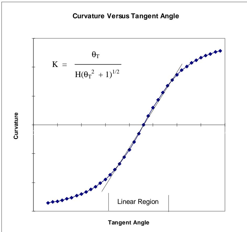
**Figure 8. Curvature versus tangent angle.** The relationship is linear within a range around zero, thus the relationship between chest angle and lumbar curvature is expected to be linear.
