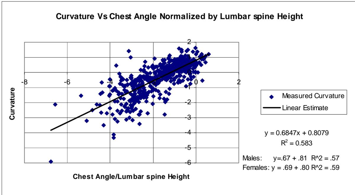
**Figure 16b** Curvature Versus Chest Angle Normalized by Lumbar Height. Units are radians/spinal height and radians/lumbar spine height, respectively.
