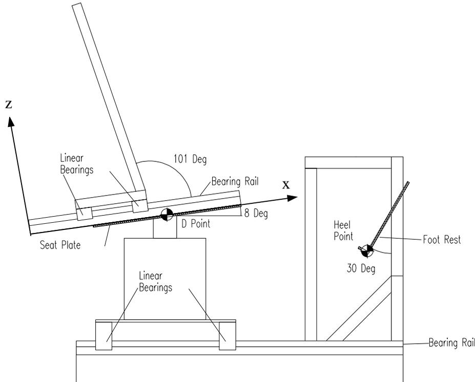
**Figure 5. Simulated drive posture measurement station.**
