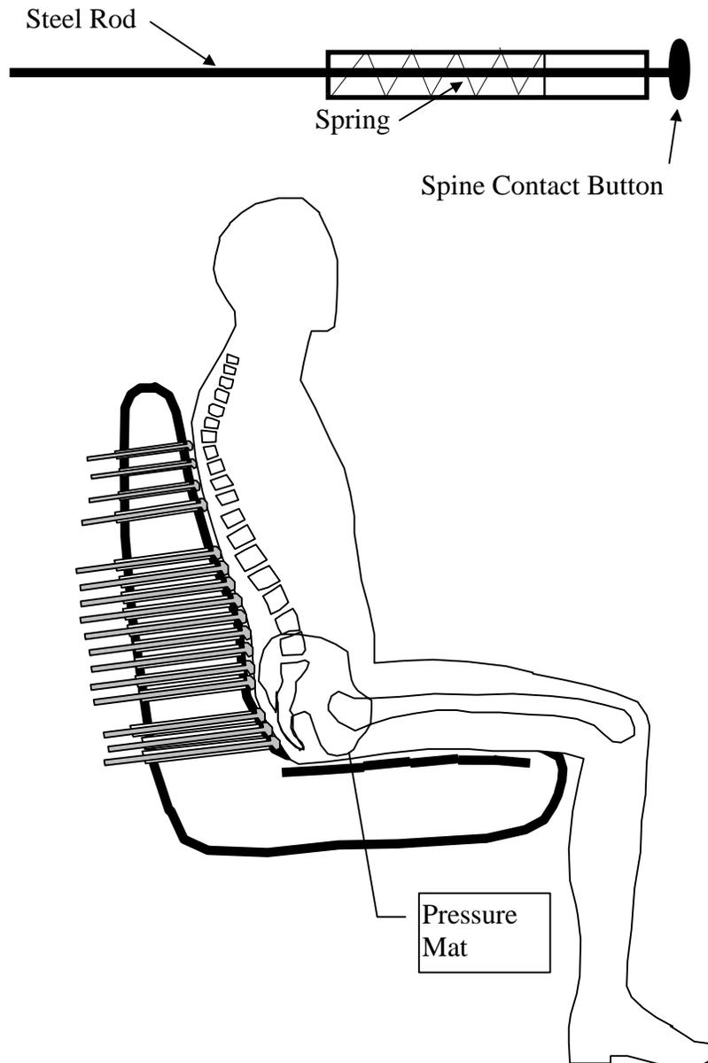
**Figure 4. Measuring Spine Contour using Spine Displacement Transducers (SDT).**
