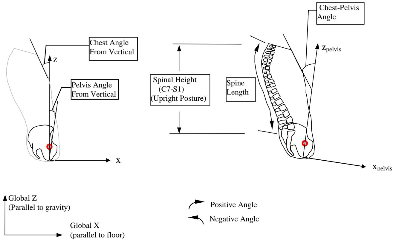
**Figure 6 Pelvic coordinate system, chest angle, spinal height and spinal length.**
