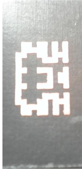
Figure 4.6. Prototype of a single element fabricated through photolithography.
