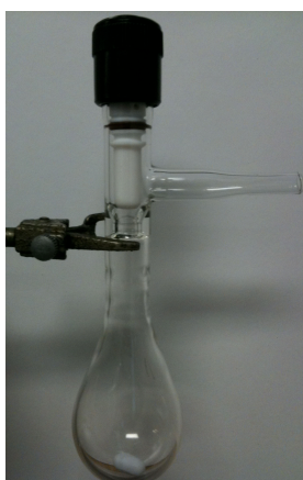
Figure 2.26 The Schlenk flask was prepared from a single-necked 25 mL pear-shaped flask that had its 14/20 glass joint replaced with a high vacuum threaded Teflon valve.
