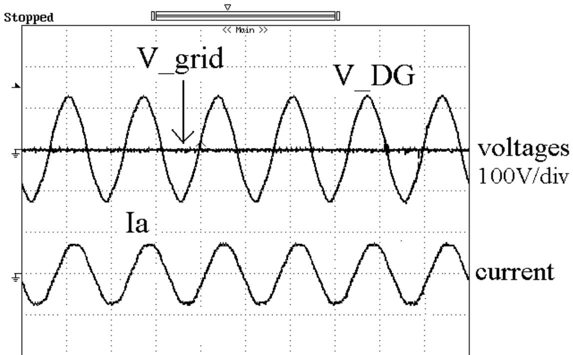
Fig. 5. 20 Line to line voltages and phase currents during intentional islanding operation
