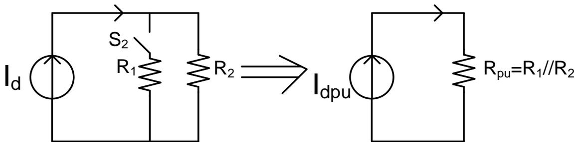
**Fig. 5. 9 System in per unit to implement load shedding**
