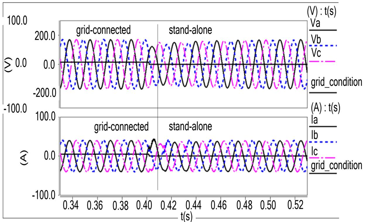
**Fig. 5. 14 From grid-connected to stand-alone operation without severe transients**
