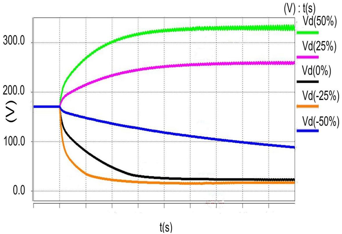
**Fig. 5. 6 Voltage Transients under various Active Power Differences**
