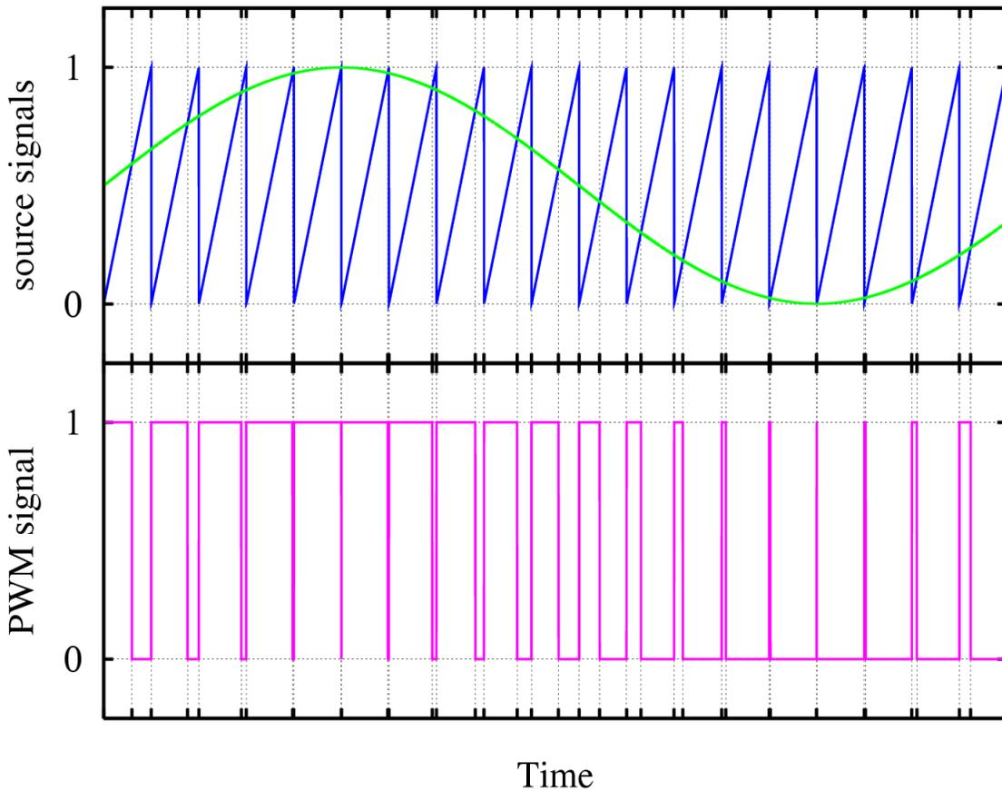
**Fig. 3. 4 PWM Operation of the Bridge**
