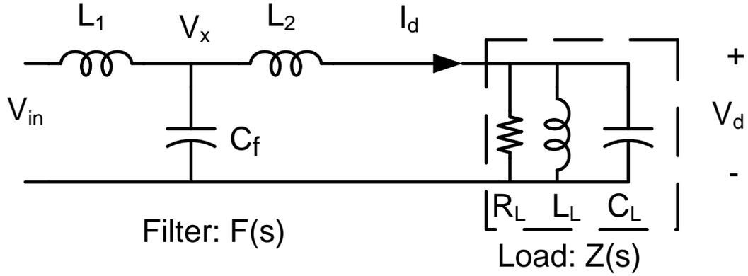
**Fig. A1. 2 LCL Filter and parallel RLC load**
