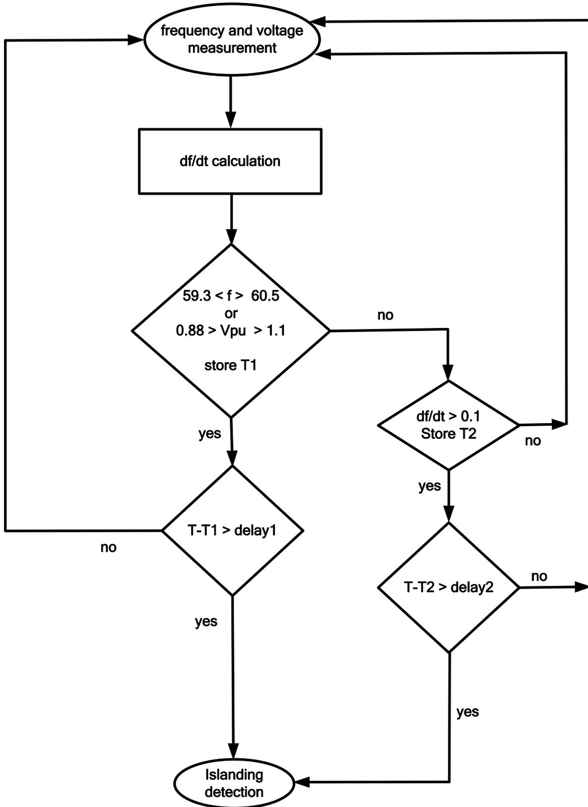
Fig. 2. 7 Proposed islanding detection algorithm [34]
