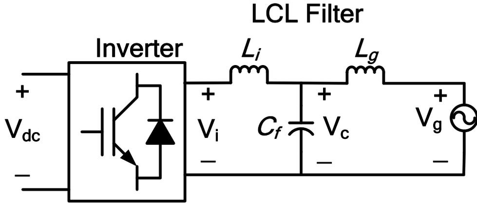
**Fig. 3. 5 LCL Filter configuration circuit**
