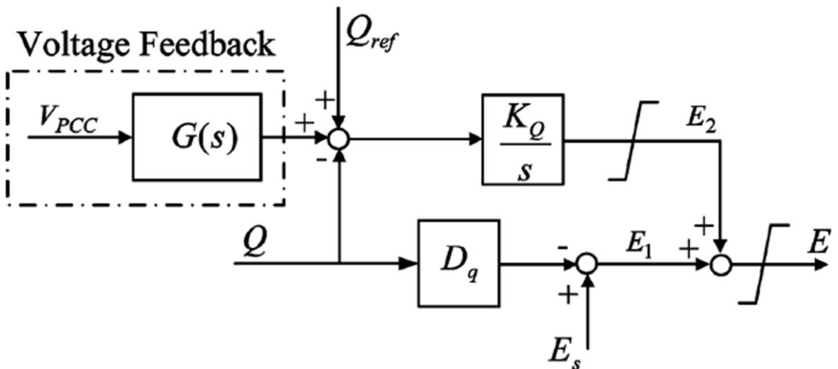
Fig. 2. 10 Block diagram of voltage control with positive feedback [35]
