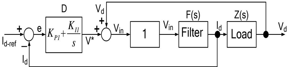
**Fig. 4. 4 Block diagram of the current controlled inverter**
