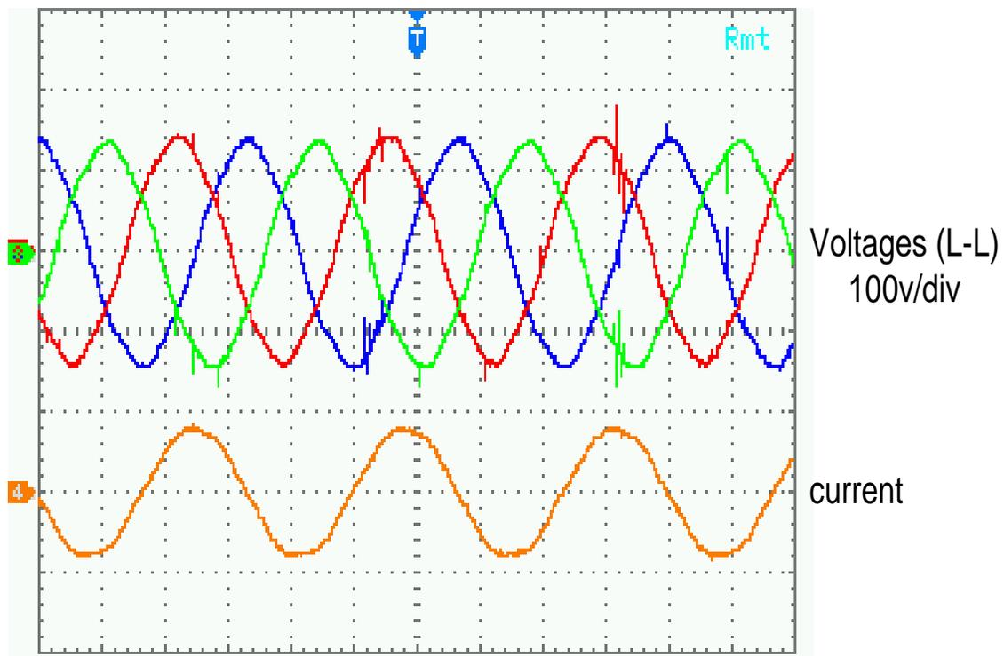
Fig. 5. 21 DG line to line voltages and phase currents during intentional islanding operation
