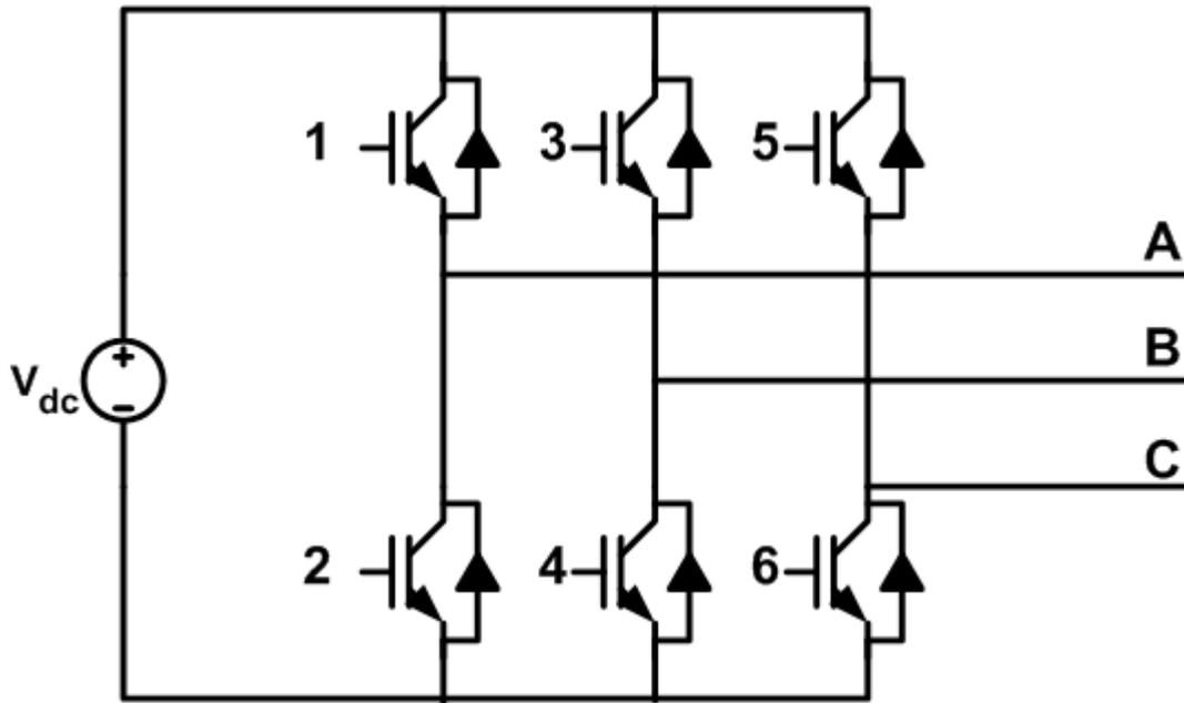
**Fig. 3. 3 DC to Three-Phase AC Inverter Diagram**
