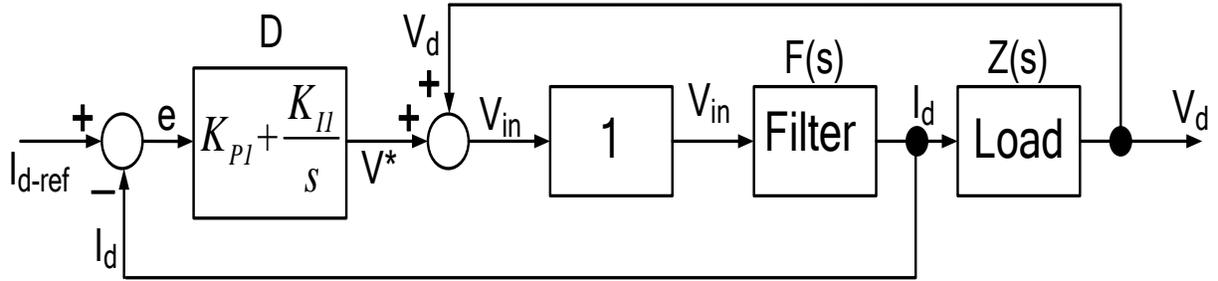
**Fig. A1. 1 Block diagram of the current controlled inverter**
