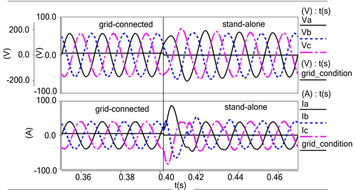
**Fig. 5. 13 From grid-connected to stand-alone operation with severe transients**
