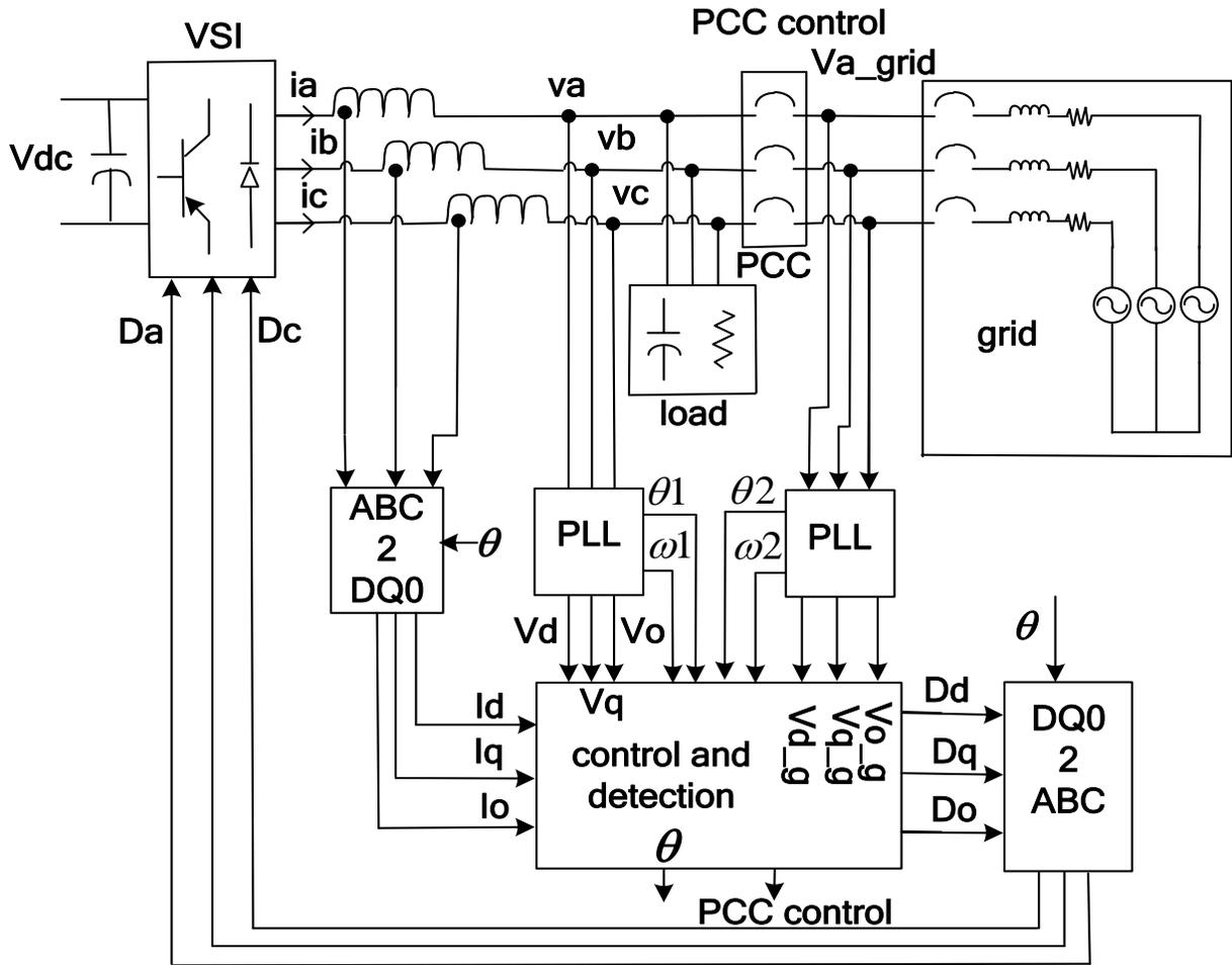
**Fig. 2. 4 System configuration for simulated and experimental results [32-33]**
