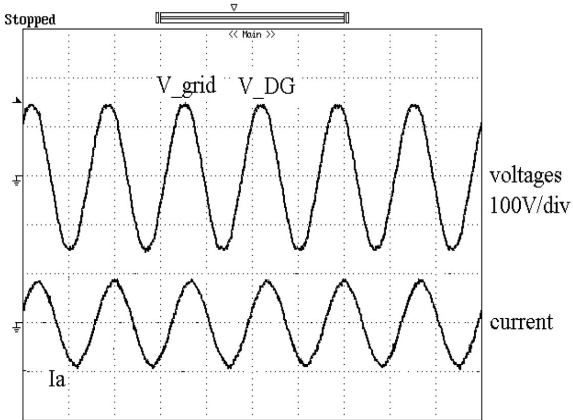
**Fig. 4. 10 Line to line voltages and phase current during grid-connected operation**
