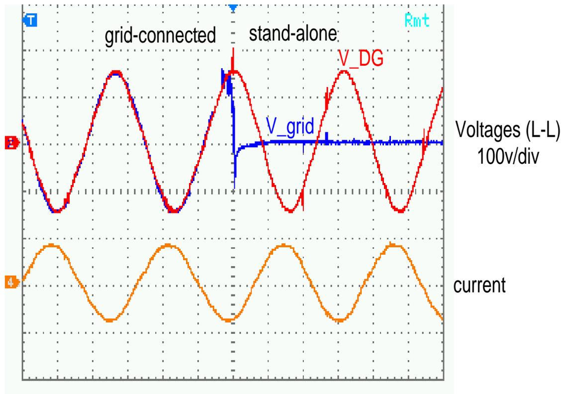
**Fig. 5. 19 Transition from grid-connected to intentional islanding operation without severe transients**
