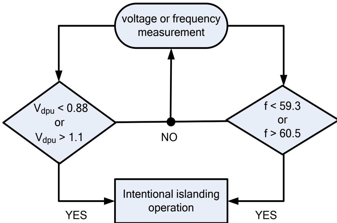
Fig. 5. 5 Islanding Detection Algorithm
