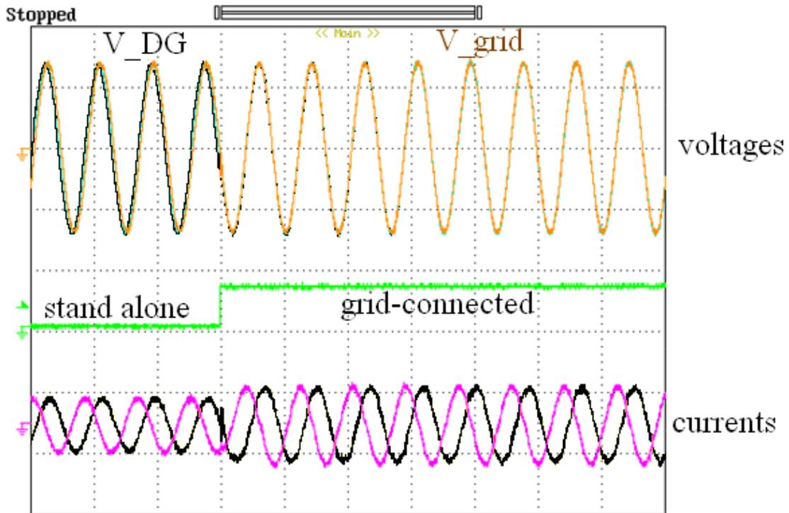
**Fig. 4. 11 Transition from stand-alone to grid connected operation**
