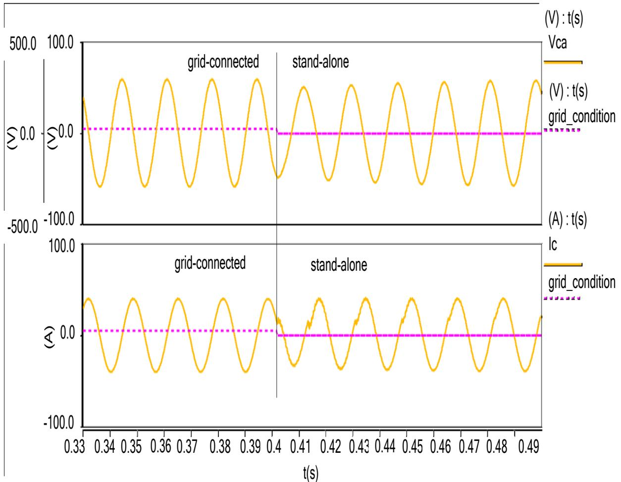
**Fig. 5. 15 From grid-connected to stand-alone operation without severe transients**
