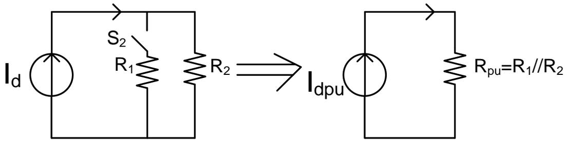
**Fig. A2. 1 System to implement load shedding**
