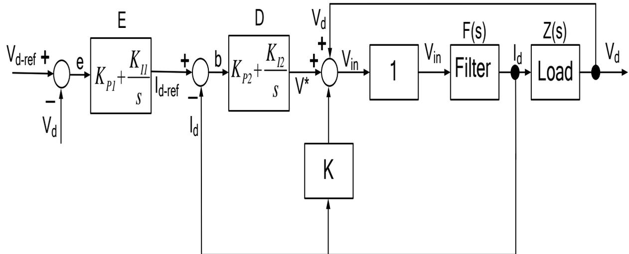
**Fig. 5. 11 Block diagram of the voltage controlled inverter**
