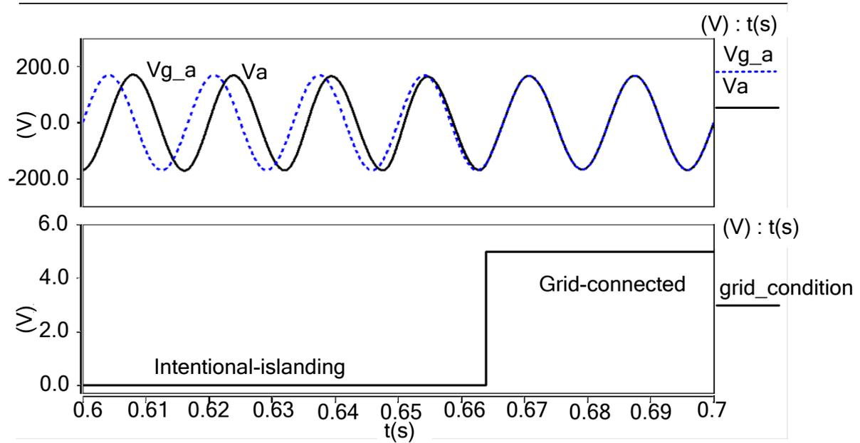
**Fig. 4. 8 Synchronization for grid re-connection**
