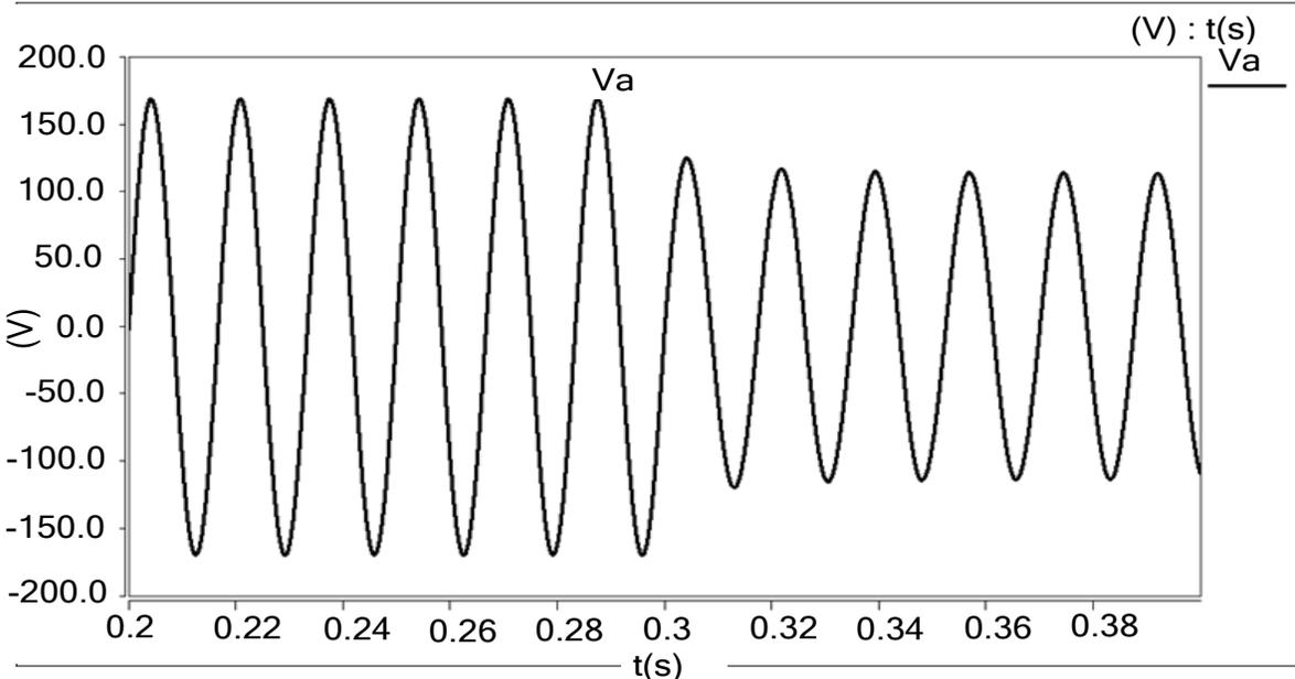
**Fig. 5. 16 Phase voltage  $V_a$  without load shedding algorithm**
