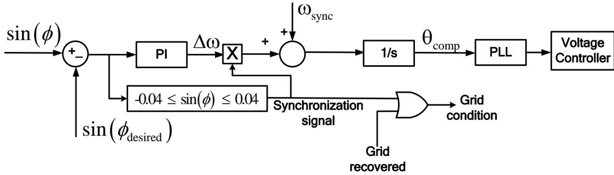
**Fig. 4. 3 Synchronization controller**
