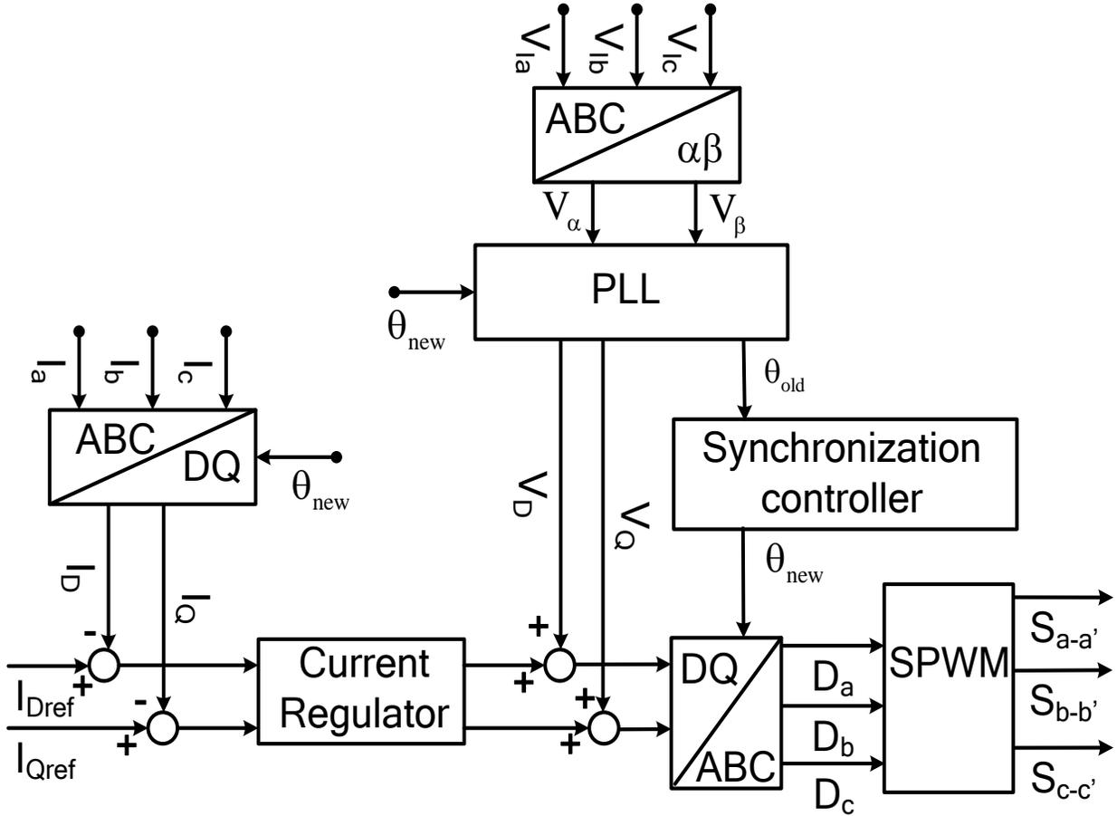
**Fig. 4. 2 Block diagram of the current controller for grid-connected**
