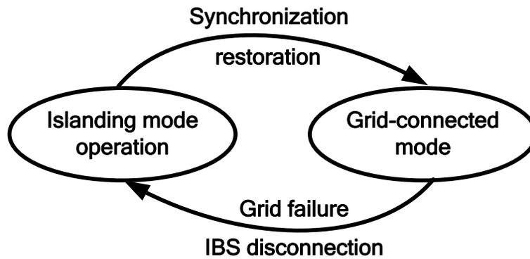
Fig. 2. 15 Flowchart diagram of the modes of the VSI [3]
