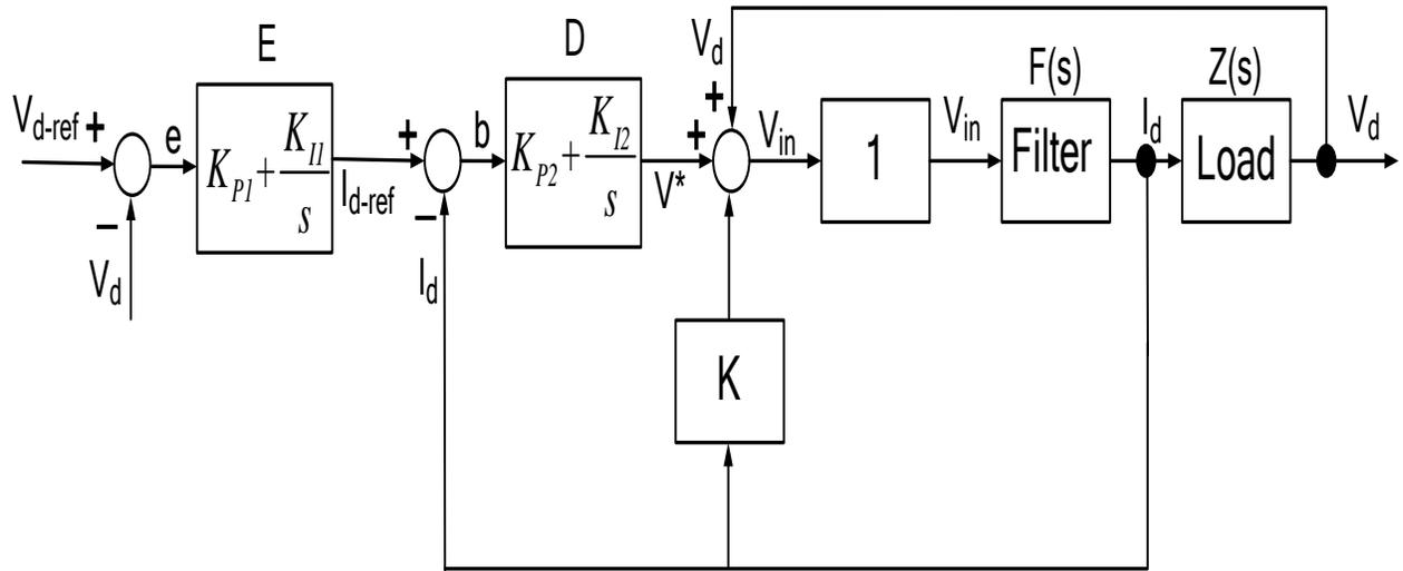
**Fig. A3. 1 Block diagram of the voltage controlled inverter**
