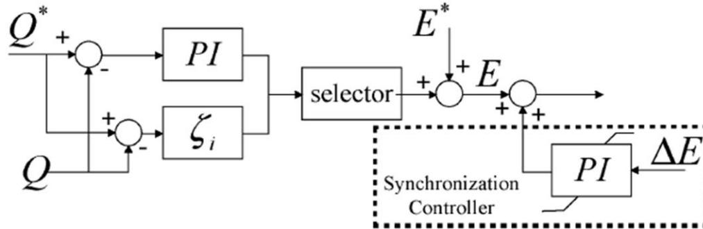
Fig. 2. 2 Reactive power compensator with synchronization function [31]
