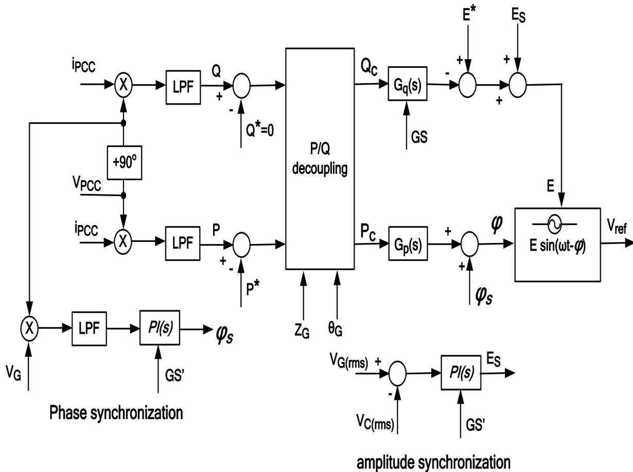
Fig. 2. 16 Block diagram of the whole proposed controller using the synchronization control loops [3]
