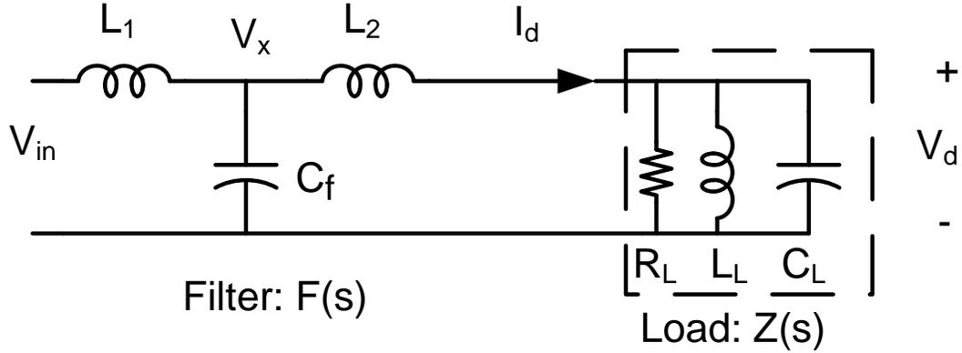
**Fig. 4. 5 LCL Filter and parallel RLC load**
