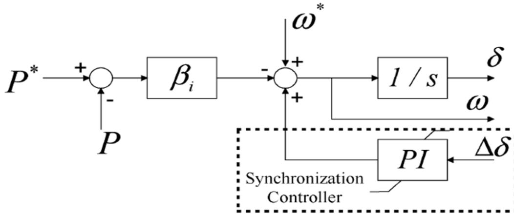
Fig. 2. 1 Real power compensator with synchronization function [31]
