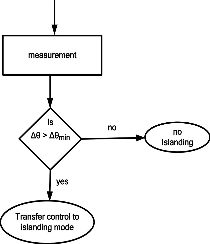
Fig. 2. 13 Islanding-detection scheme [39]
