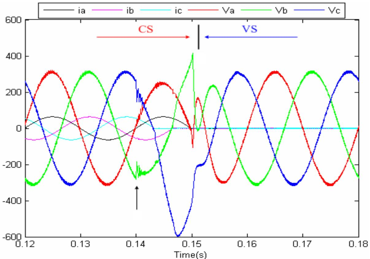
**Fig. 5. 1 Simulation waveforms of load voltages and grid currents during the grid disconnection [38]**
