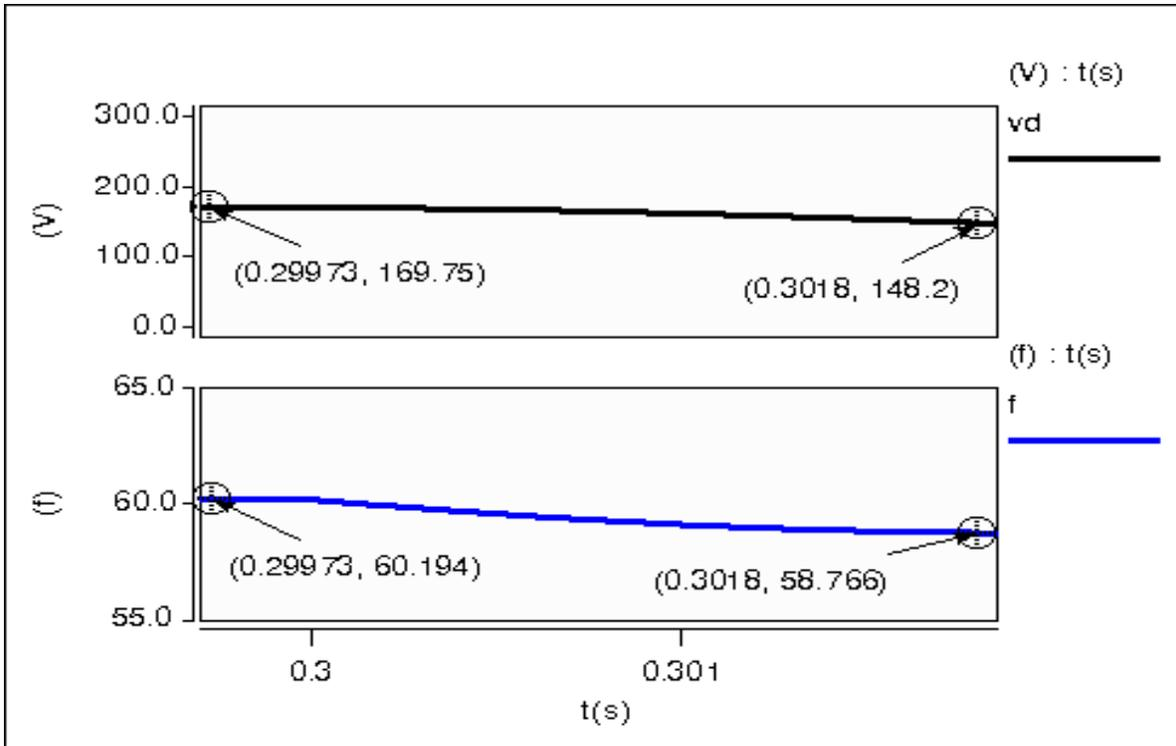
Fig. 5. 4 Voltage or frequency change at grid disconnection
