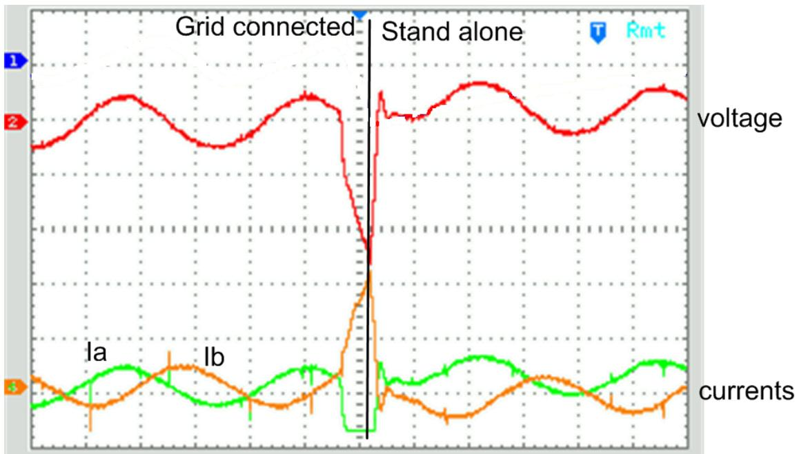
**Fig. 5. 18 Transition from grid-connected to stand-alone operation with severe transients**
