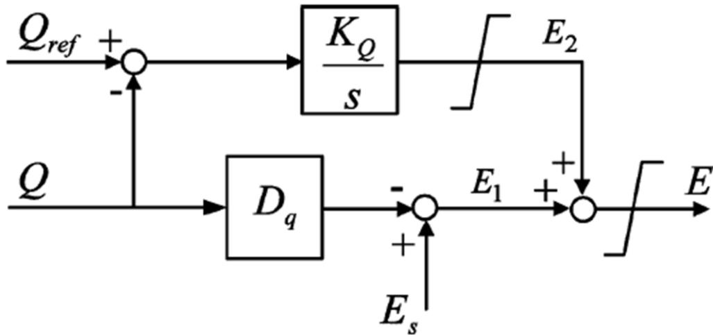
Fig. 2. 9 Block diagram of voltage control [35]
