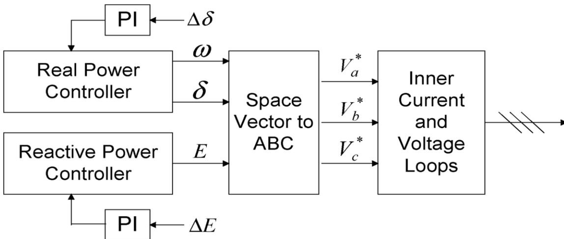
Fig. 2. 3 Overview of proposed unified controller [31]
