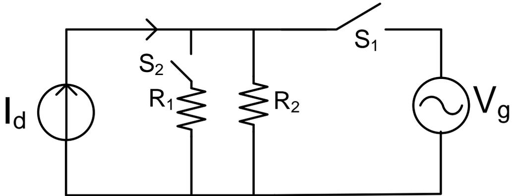
**Fig. 5. 8 System to implement load shedding**
