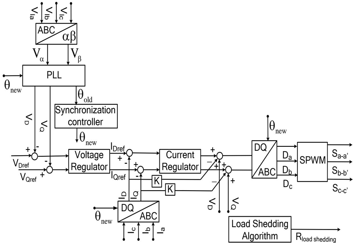
**Fig. 5. 10 Voltage controlled inverter**
