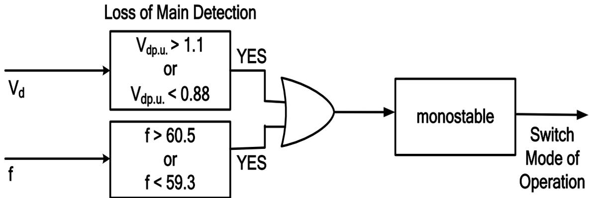
**Fig. 5. 3 Loss of Main Detection**
