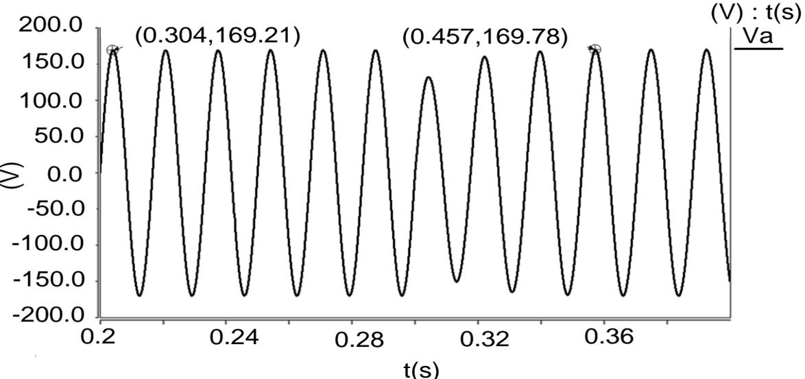
**Fig. 5. 17 Phase voltage  $V_a$  with load shedding algorithm**
