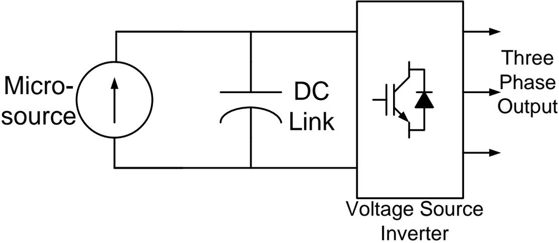
**Fig. 3. 2 Typical diagram of micro-source generation system**
