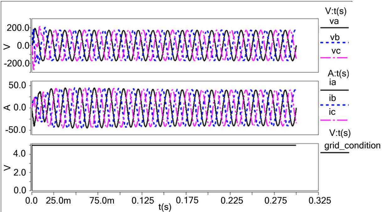
**Fig. 4. 7 Phase voltages and currents during grid-connected operation**
