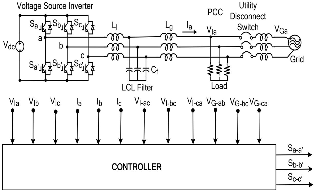
**Fig. 4. 1 Schematic diagram of the grid-connected inverter system**
