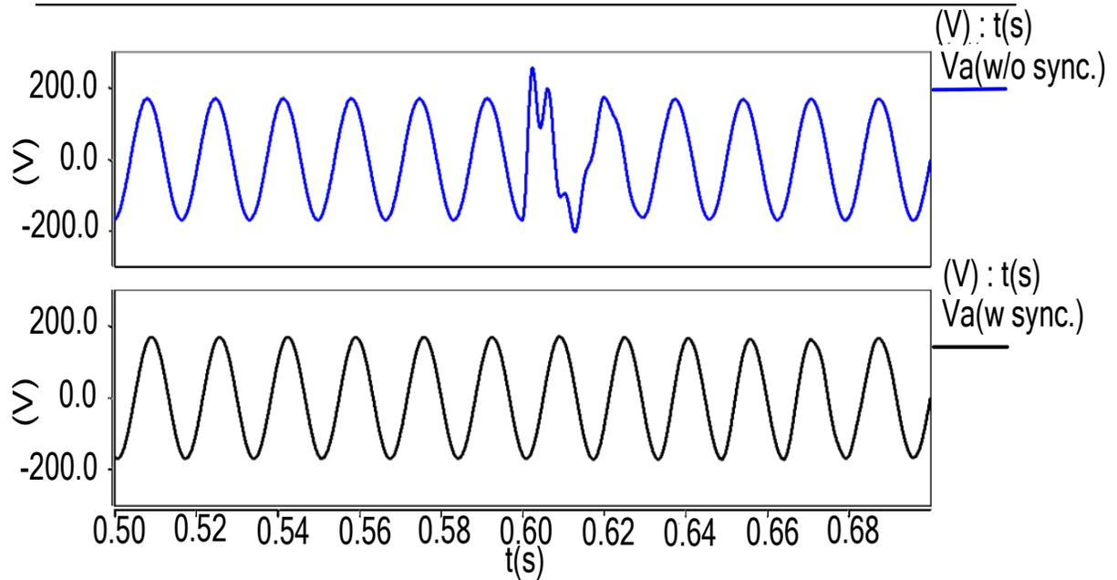
**Fig. 4. 9 Phase voltage without (top) and with (bottom) synchronization**
