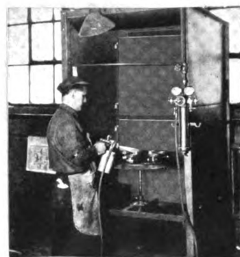
Proper method for lighting small spray booths. Note baffles for protecting lamp unit from spray residue.
