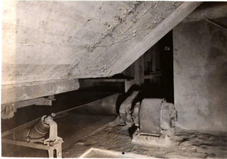
Figure No. 45. Totally-Enclosed-Fan Ventilated Motor Employed to Drive Receiving Belt under Car Shed.
