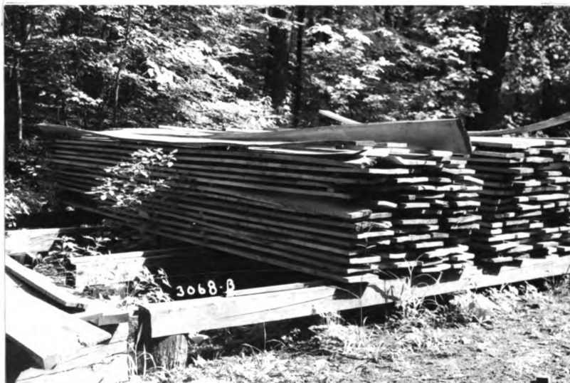
Figure No. 43 Improperly piled lumber.
