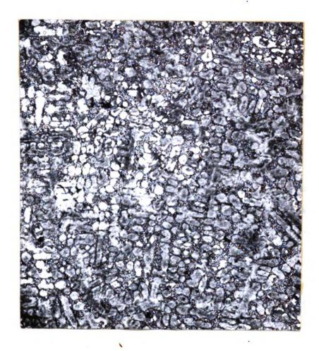
Photomicrograph 3- 2% Nital etch. Showing abnormal structure after Magnesium inoculation.
