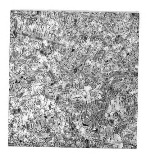
Photomicrograph 1- 2% Nital etch. Showing Abnormal structure with type D graphite. (Blank for Magnesium inoculation).
