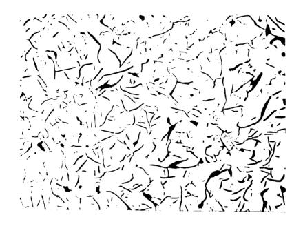
Photomicrograph 2- 2% Nital etch. Showing normal graphite pattern.
