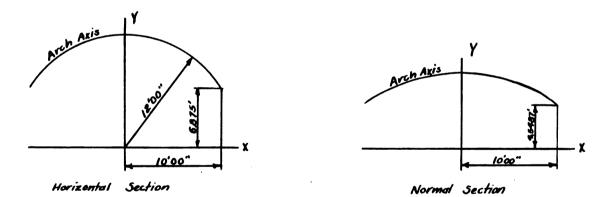
In the horizontal section through the arch when x = 4 or -10, y = 6.875. Since the slope of the face of the dam is  $\frac{15}{17}$ , when  $x_{-} \neq$  or -10,  $y = 6.875 \times \frac{15}{\sqrt{15^{2} \neq 17^{2}}} = 4.5487$  in section normal to face of the dam and the semiminor axis of the ellipse is  $12 \times \frac{15}{\sqrt{15^{2} \neq 17^{2}}} = 7.9395$ . The general formula for an ellipse is  $\frac{x^{2}}{x^{2}} \neq \frac{y^{2}}{b^{2}} = 1$
