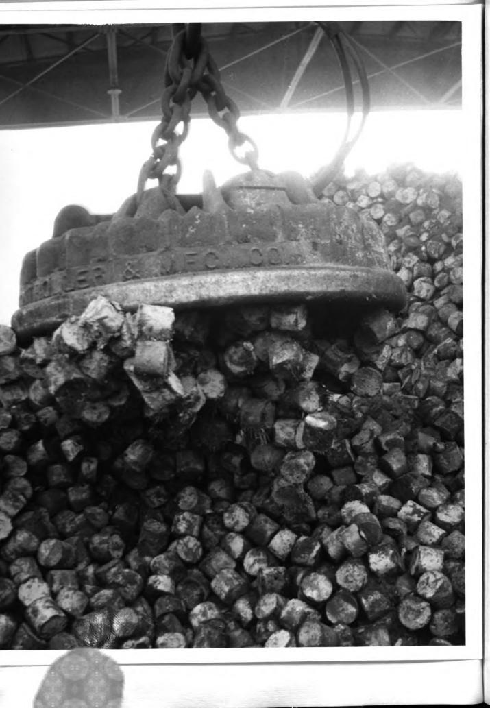
Magnet picking up briquetted borings from the pile.
