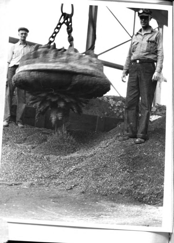
Magnet picking up borings from the pile.
