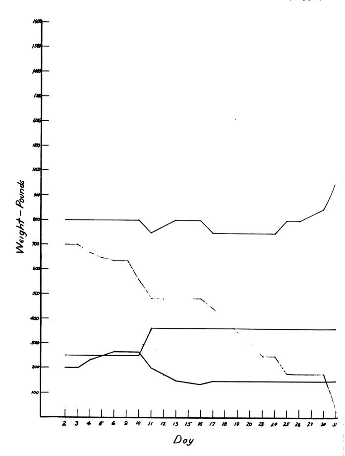
In order to increase the briquetted boring percentage and keep analysis in line, it was soon found necessary to decrease the plate steel.
