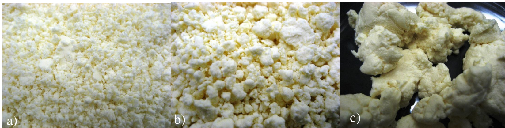
Figure 3.3. Photographs of the EWP-GLY-water mixtures with GLY contents of a) 35 %, b) 40 %, and c) 45 % and 0.48 water activity (area of 2 cm x 1.5 cm).
