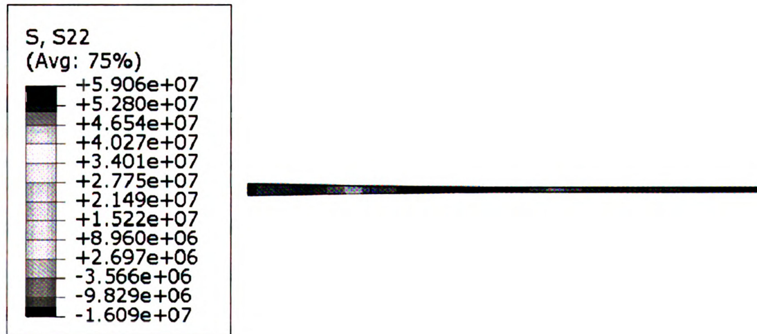
(b) Nominal inter-laminar normal stress in the cohesive zone
