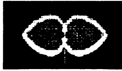
(a) Predicted delamination at bottom 90/0 interface
