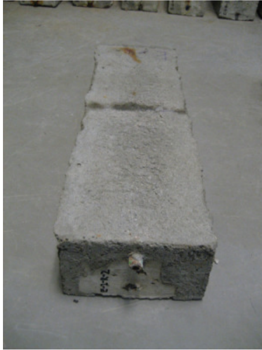
Figure 2.16: Specimen with Shallow Concrete Overlay
