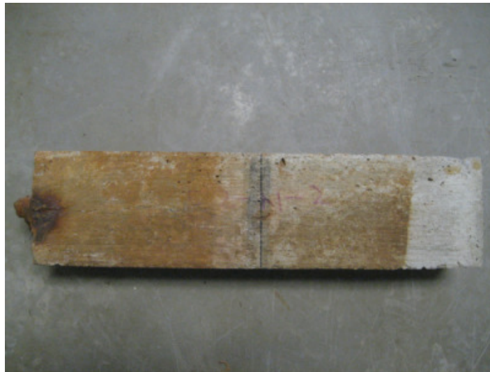
Figure 2.11: Specimen after Level 2 Corrosion
