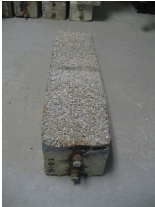
Figure 2.14: Specimen Repaired with Epoxy Overlay
