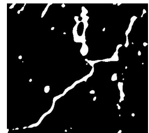
Figure B.10: B-3-N X-Ray Image and Crack after Applying Threshold
