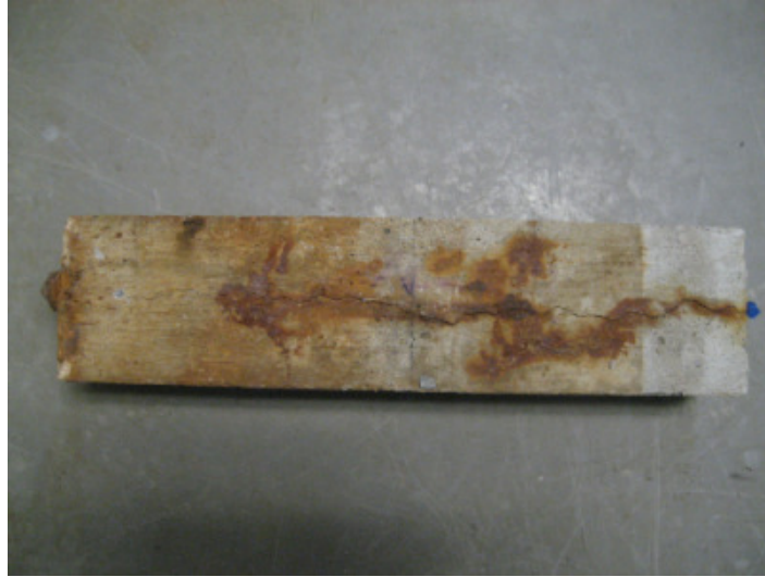
Figure 2.12: Specimen after Level 3 Corrosion
