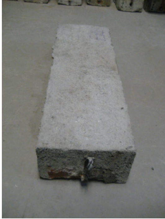
Figure 2.19: Specimen with Deep Concrete Overlay
