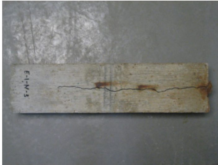
Figure 2.10: Specimen after Level 1 Corrosion
