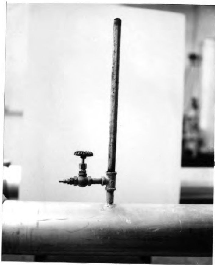
Fig. 6 Close-up of piezometer tube with stop cock and manometer tube attachment fittings.
