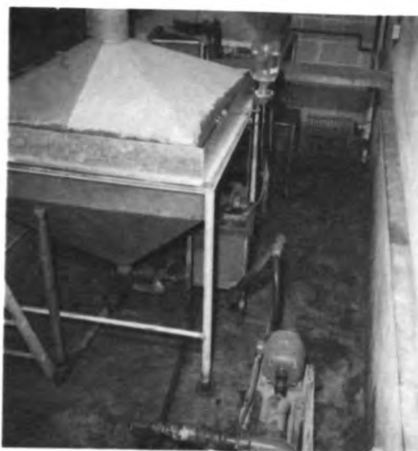
Figure 2 CYANIDE FEED AND SETTLING TANK
