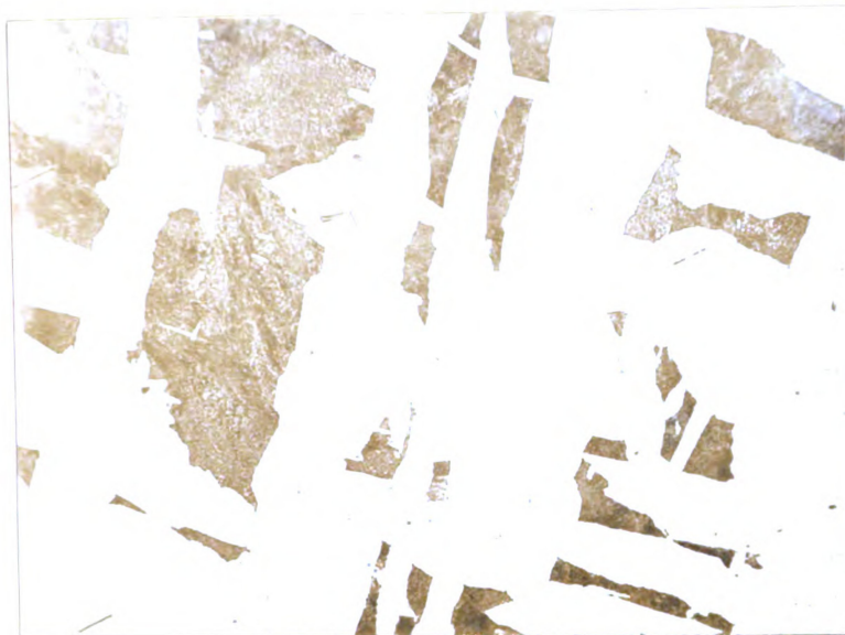
Figure 30. Sample 5431-C; picric acid etch; X 75; C - 0.16%.
