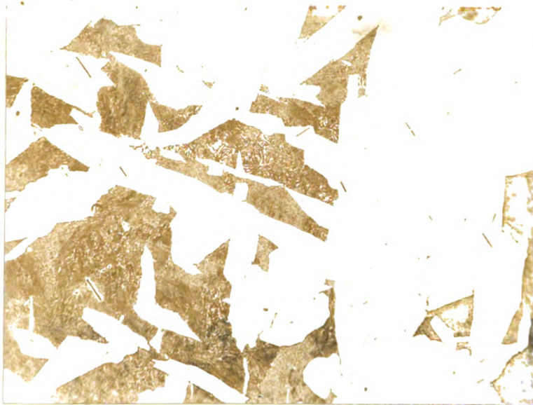
Figure 28. Sample 5431-A; picric acid etch; X 75; C - 0.19%.
