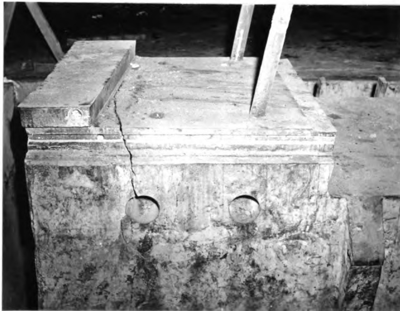
Figure 2. Typical hammer base failures.
