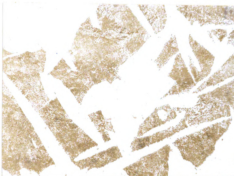
Figure 25. Sample 7331-A; picric acid etch; X 75; C - 0.19%.
