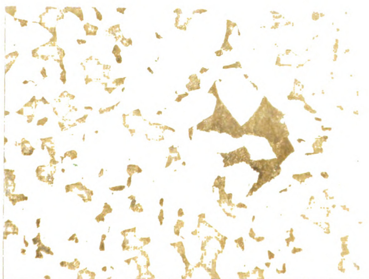
Figure 26. Sample 7331-A; picric acid etch; X 75; C - 0.49%.
