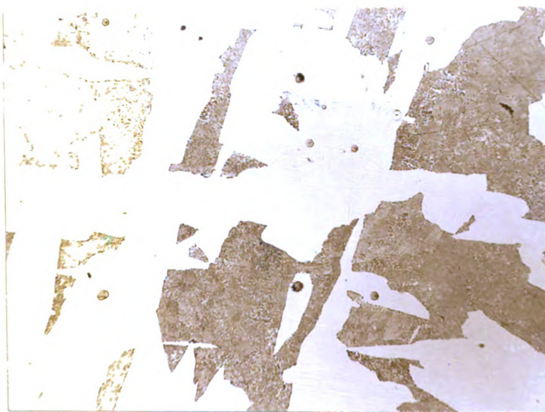
Figure 22. Sample 7449; picric acid etch; X 75; C - 0.20%.
