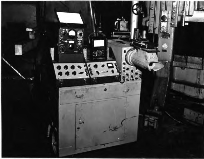
Figure 4. Strain gage instrumentation.
