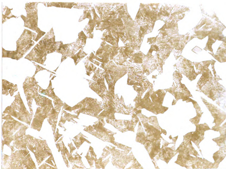
Figure 29. Sample 5431-B; picric acid etch; X 75; C - 0.33%.
