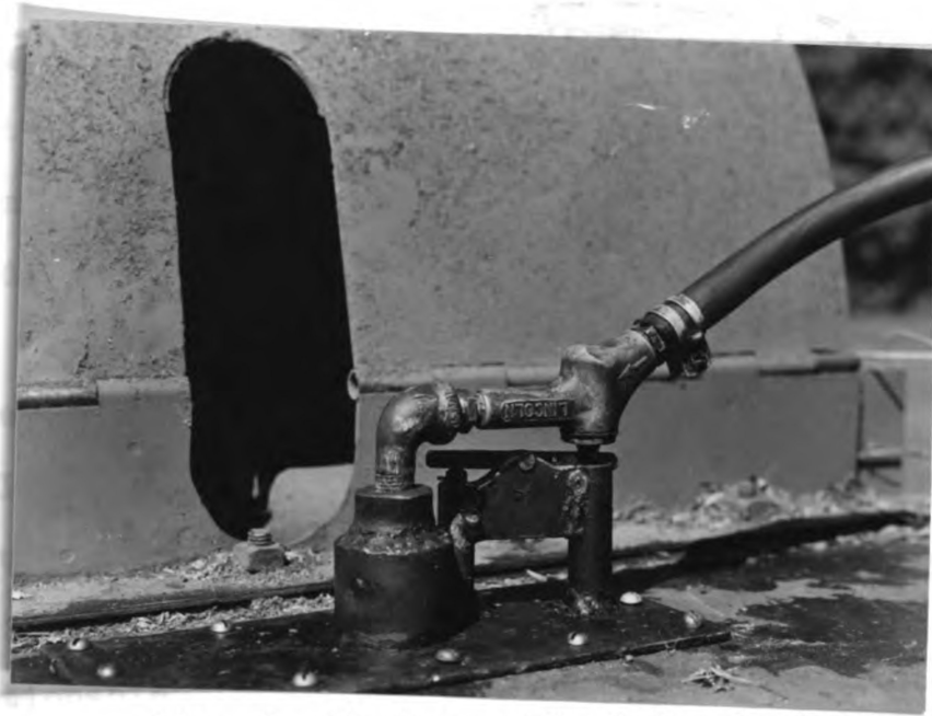
Fig. 9. Single nozzle bale chamber spray unit.
