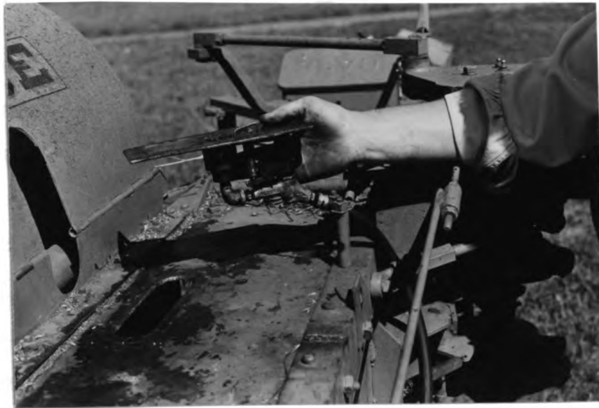
Fig. 10. Underside of bale chamber spray unit. At each stroke of the plunger the wedge is forced up, shutting off the spray.
