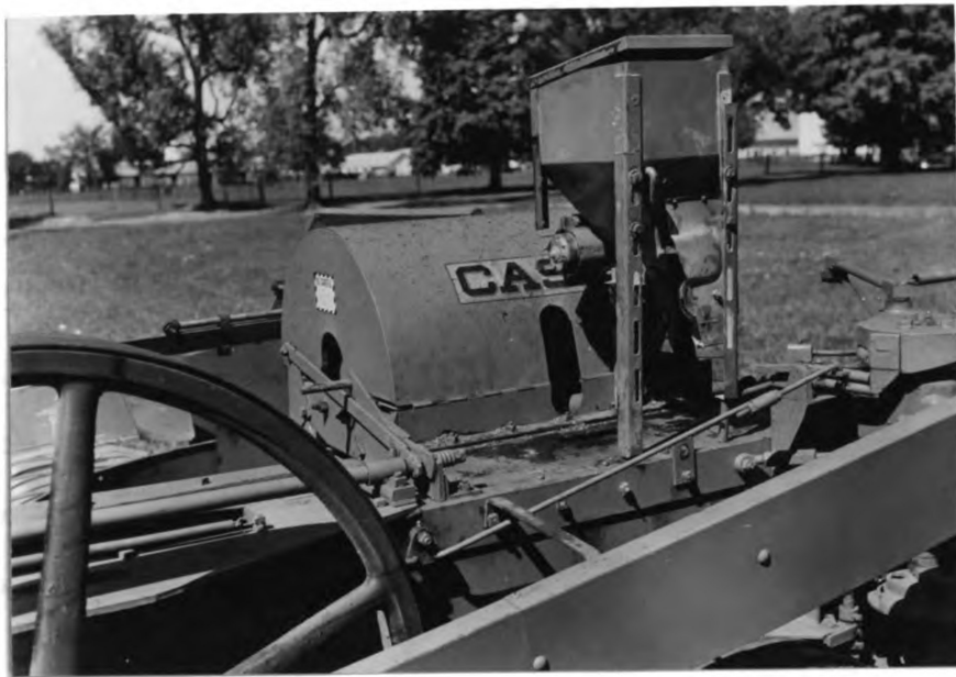
Fig. 7. Crop preservative dust dispenser mounted on baler.
