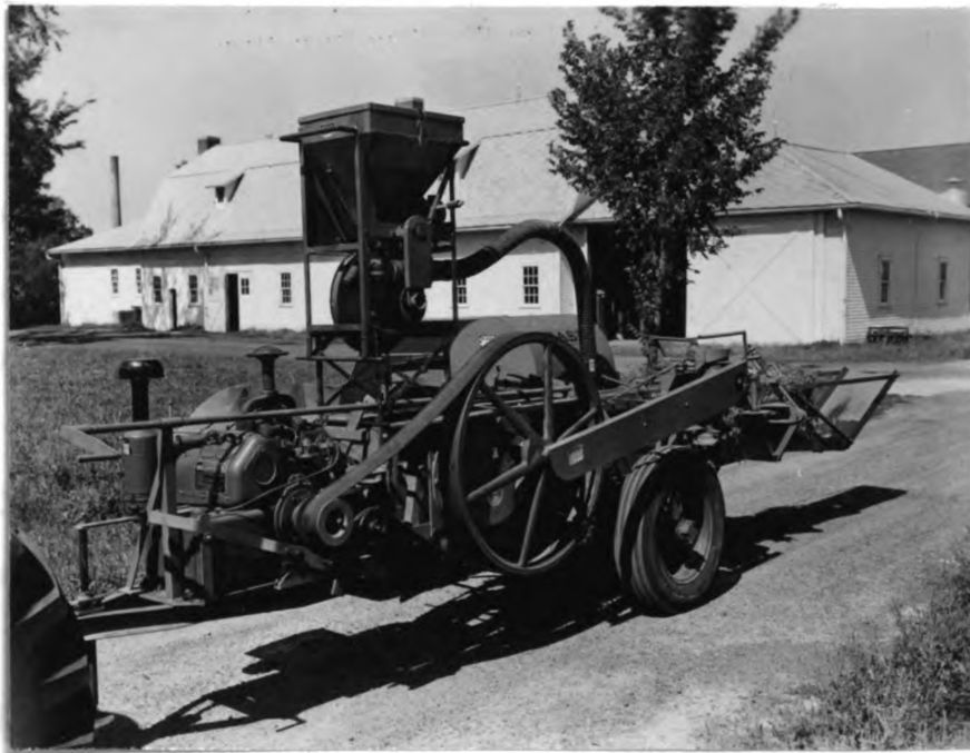
Fig. 8. Greenhouse duster mounted on baler.
