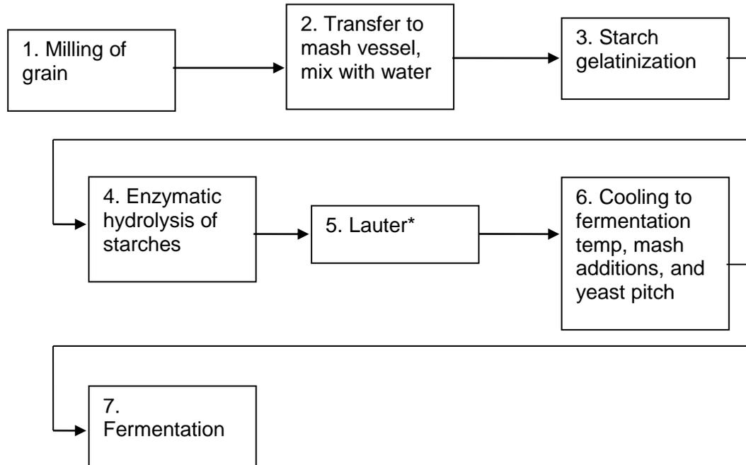
Figure 1: Grain processing flow chart
