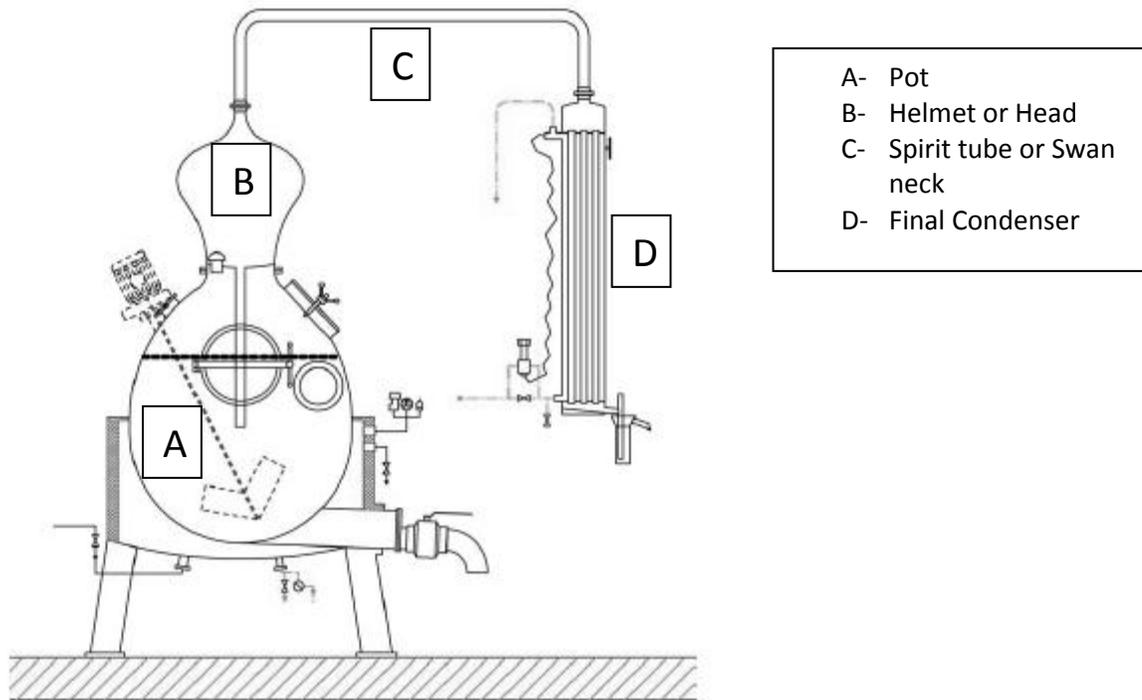
Figure 2: Modern steam jacket style, alambic distillery (Figure reproduced courtesy of Christian Carl Ing. GmbH)
