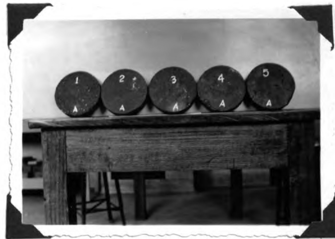
Fig. 4. Coarse Sand Mix--alternate freezing & thawing for 5 weeks.
