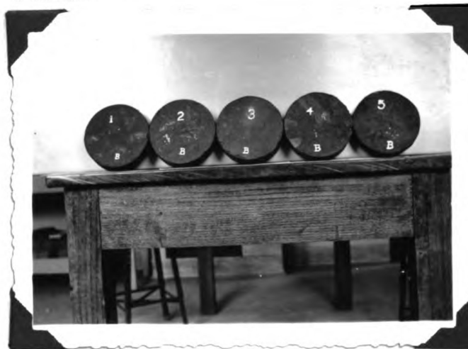
Fig. 7. Fine Sand Mix--alternate freezing & thawing for 5 weeks.
