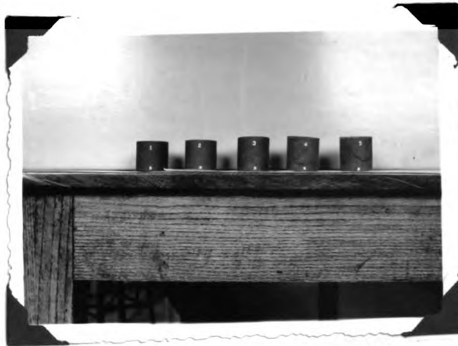
Fig. 5. Fine Sand Mix--absorption test; 14 days in water.
