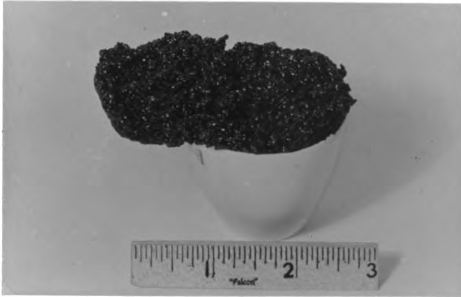
Figure 20. Biotite Granite Sample after Magma Upwelling in Vacuum at 1000^{\circ}\text{C} .
