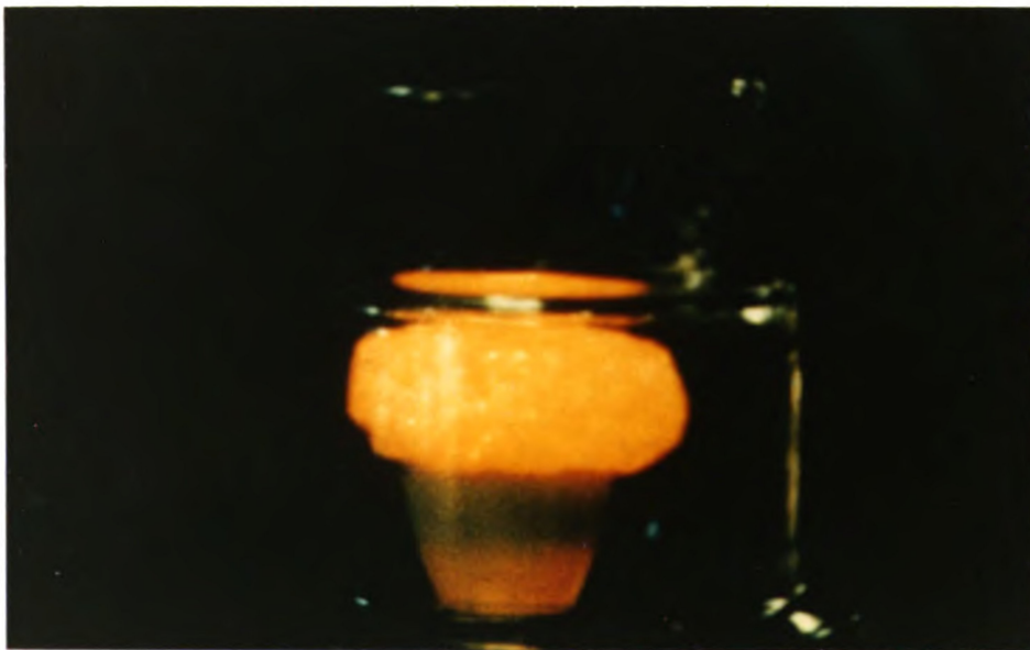
Figure 6. Second Phase of Wausau Sand Upwelling in Vacuum. Note Visible Color Temperature Increase at Base of Crucible. Time 33 seconds.
