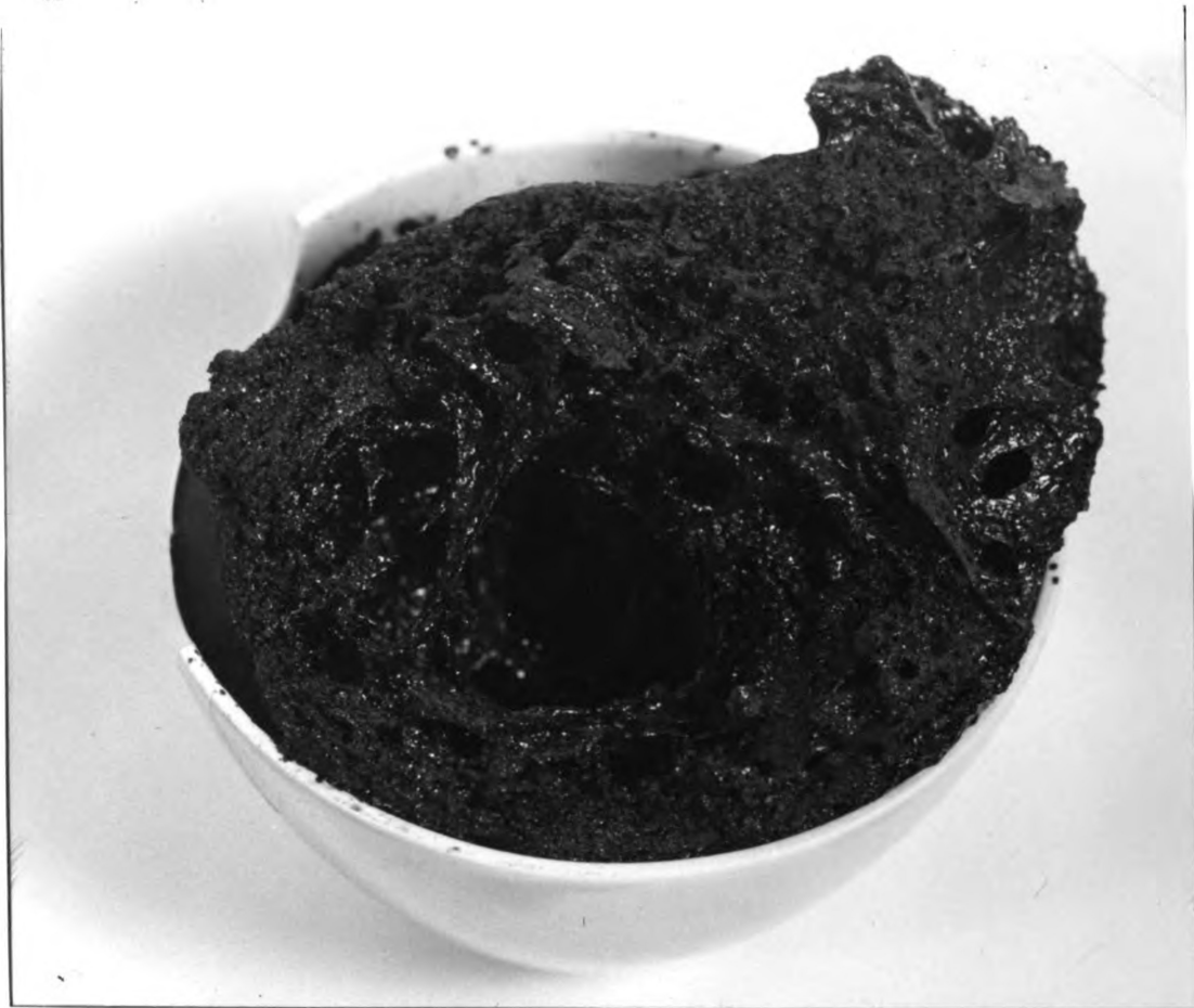
Figure 26. Basalt Sample Showing Internal Structure Formed from Melt at 1000°C Upwelled in Vacuum.
