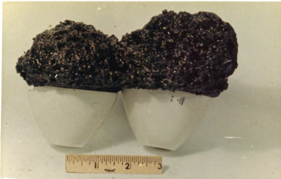
Figure 17. Basalt Sample after Rock Melt Upwelling in Vacuum at 1000° C.
