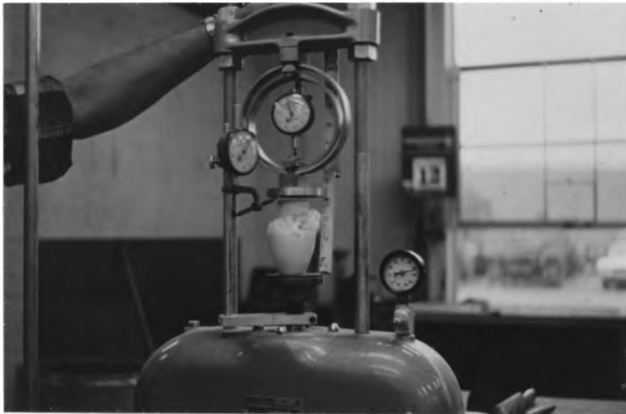
Figure 3, Bearing Strength, Unconfined Compression, Experimental Test Set Up.
