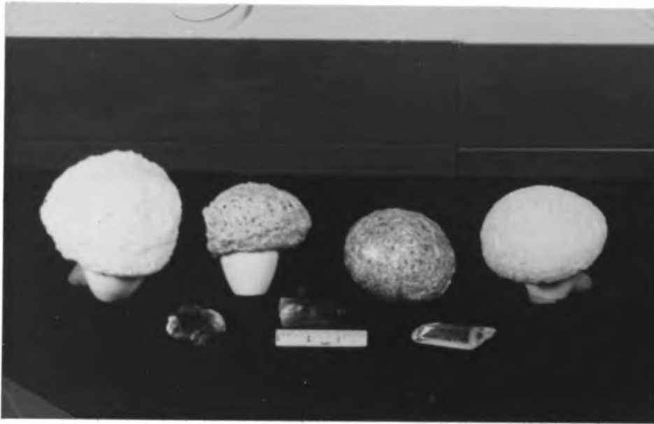
Figure 29. Radiation Discoloration of Silica
