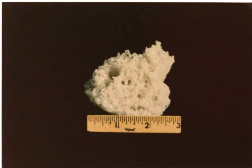
Figure 23. Wausau Sand Sample Showing Sponge Like Structure Formed from Melt at 1500^{\circ}\text{C} Upwelled in Vacuum.
