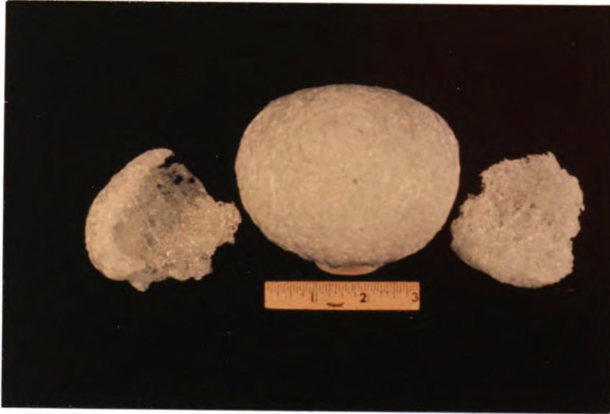
Figure 24. Flint Glass Sample Formed from Melt at 1500^{\circ}\text{C} Upwelled in Vacuum. Note "Pele's Hair" Structure on Outer Surface and Large Internal Void Area.
