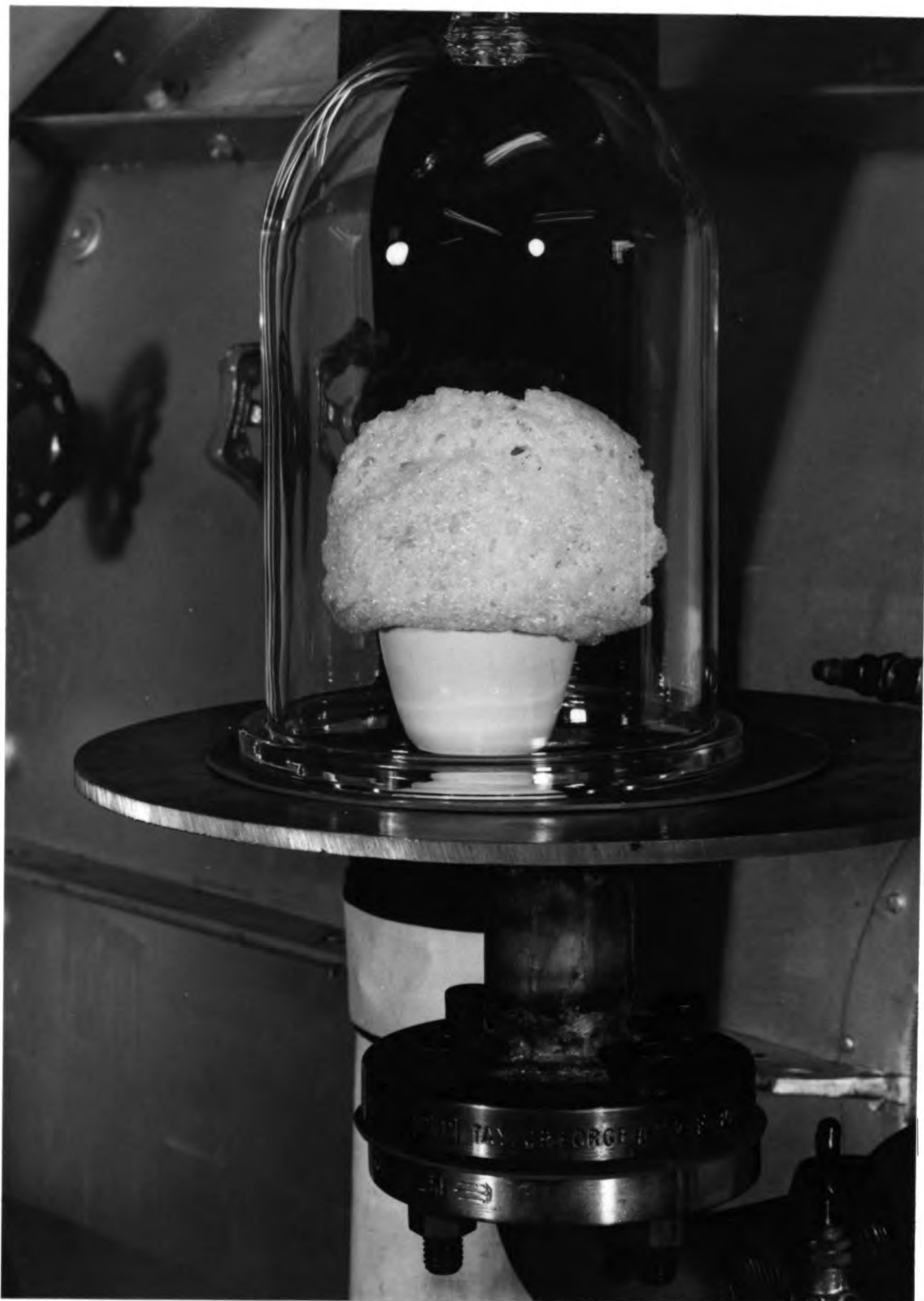
Figure 2. Bell Jar Baseplate Assembly Showing Upwelled Wausau Sand Sample Within Bell Jar and the Bell Jar - Rubber Gasket - Baseplate Seal.
