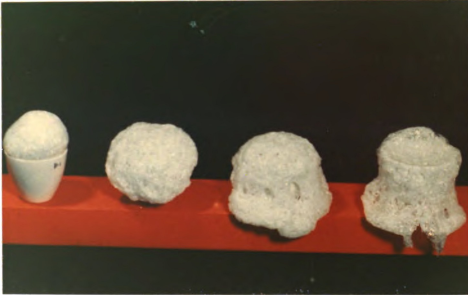
Figure 8. Wausau Sand Samples which were Upwelled in Vacuum at Different Rock Melt Temperatures.
