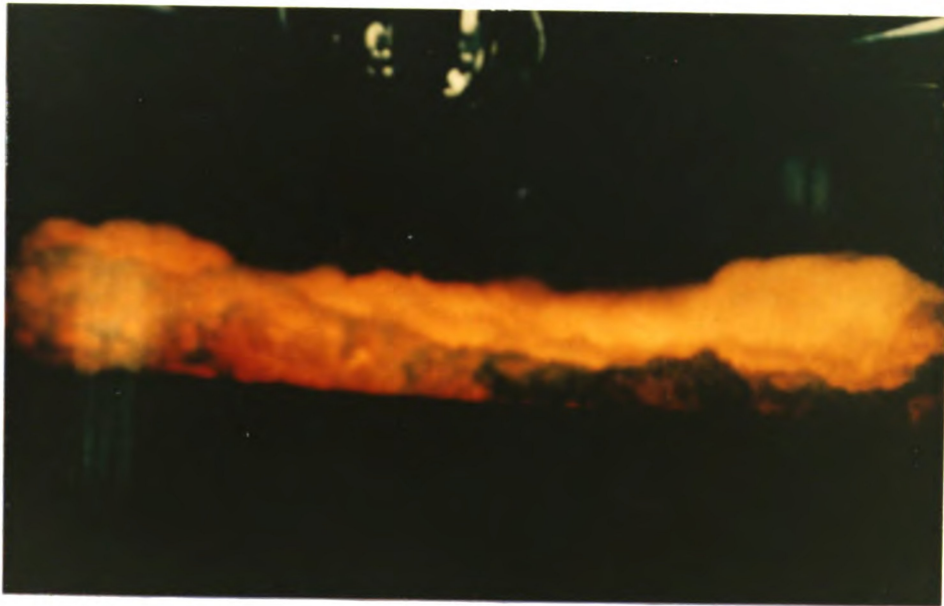
Figure 10. Vacuum Upwelled Multiple Crucible Sample, same as Figure 9, after Collapsing Due to a Partial Atmospheric Pressure Build Up Due to Rock Melt Outgassing.
