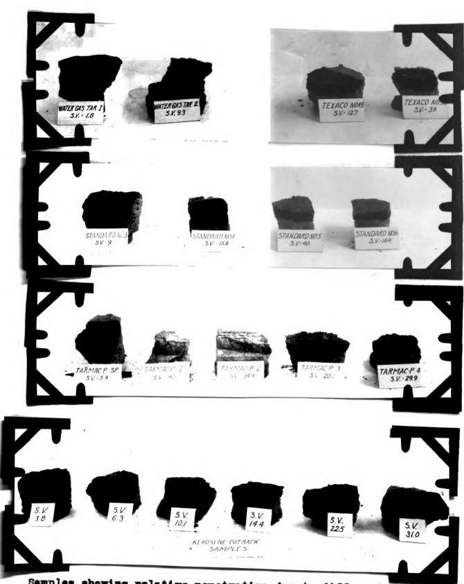
Samples showing relative penetration due to different viscosities.
