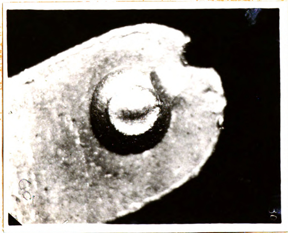
C30. Pt. #189a. 788960 impulses. Neg. Damper Spring.
