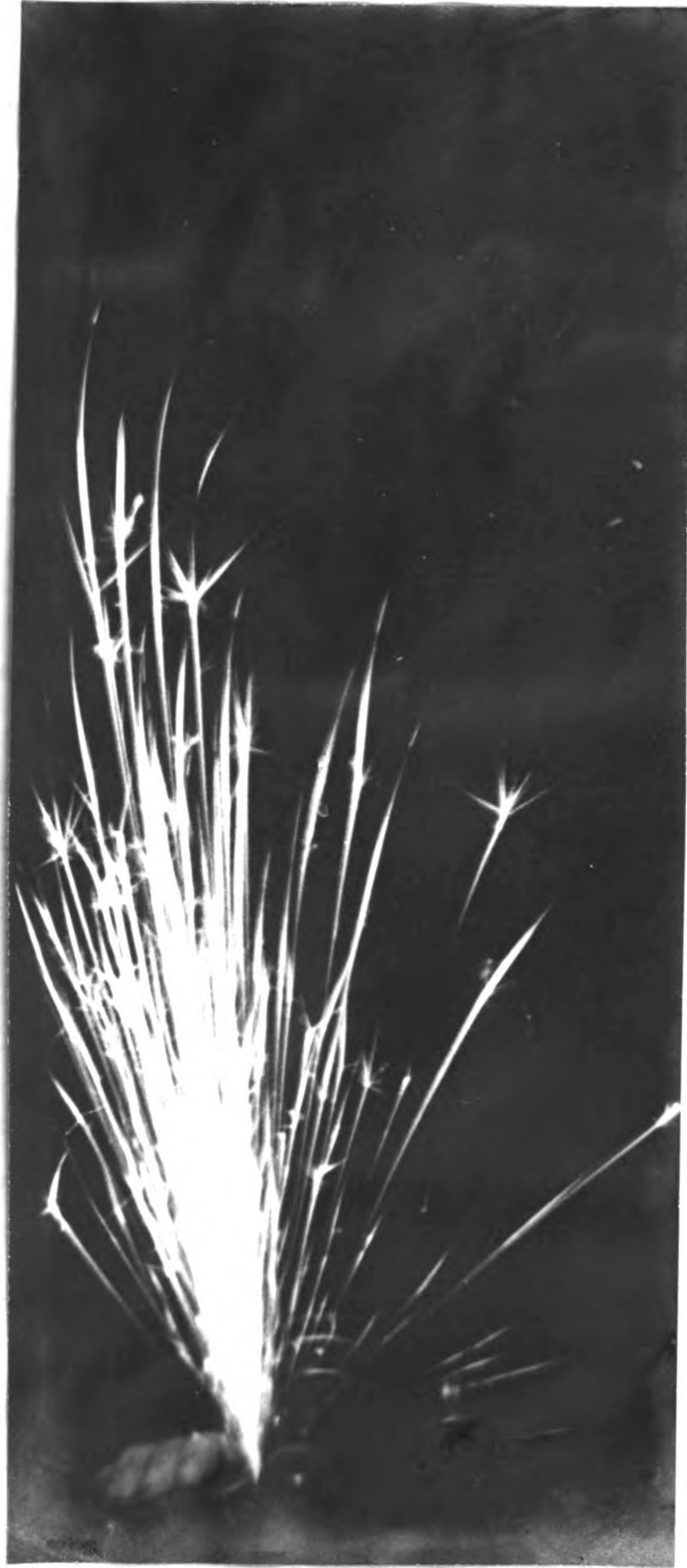
Fig. 13A - Spark streams typical of chromium-vanadium steels -
