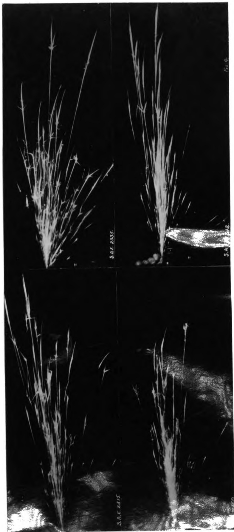
Fig. 4 - Spark streams typical of S.A.E. nickel steel
