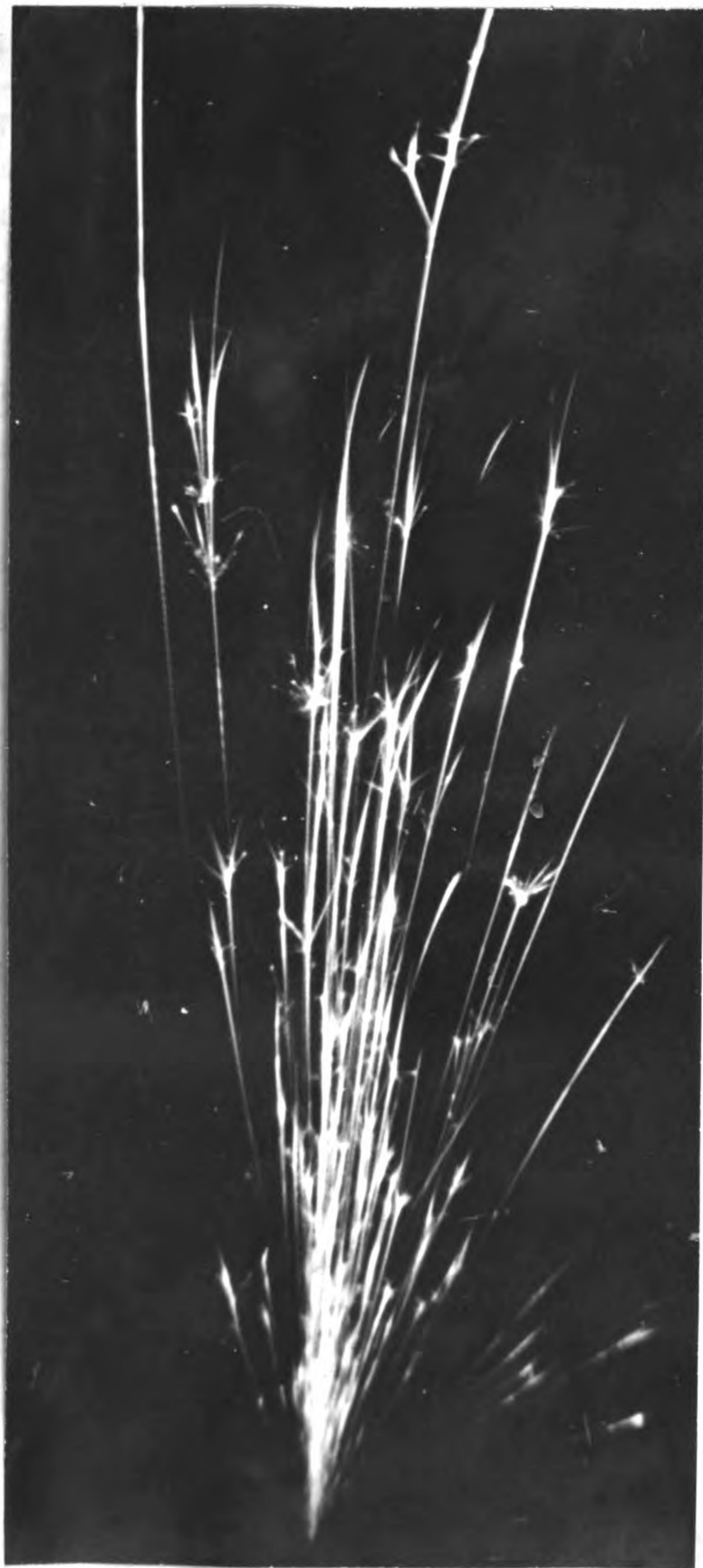
Fig. 9A - Spark streams typical of chromium-nickel steels -
