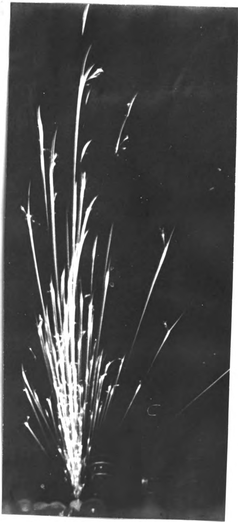
Fig. 18 - Spark streams of typical silica-manganese steel, showing jacketing effect - Type S.A.E. 9250
