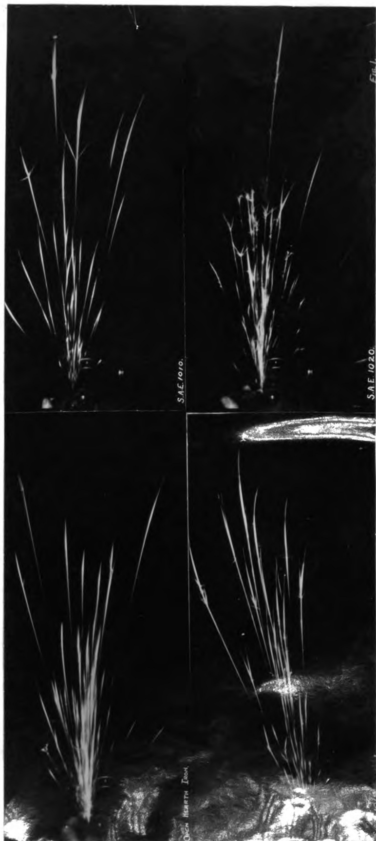
Fig. 1 - Spark streams typical of low carbon steel
