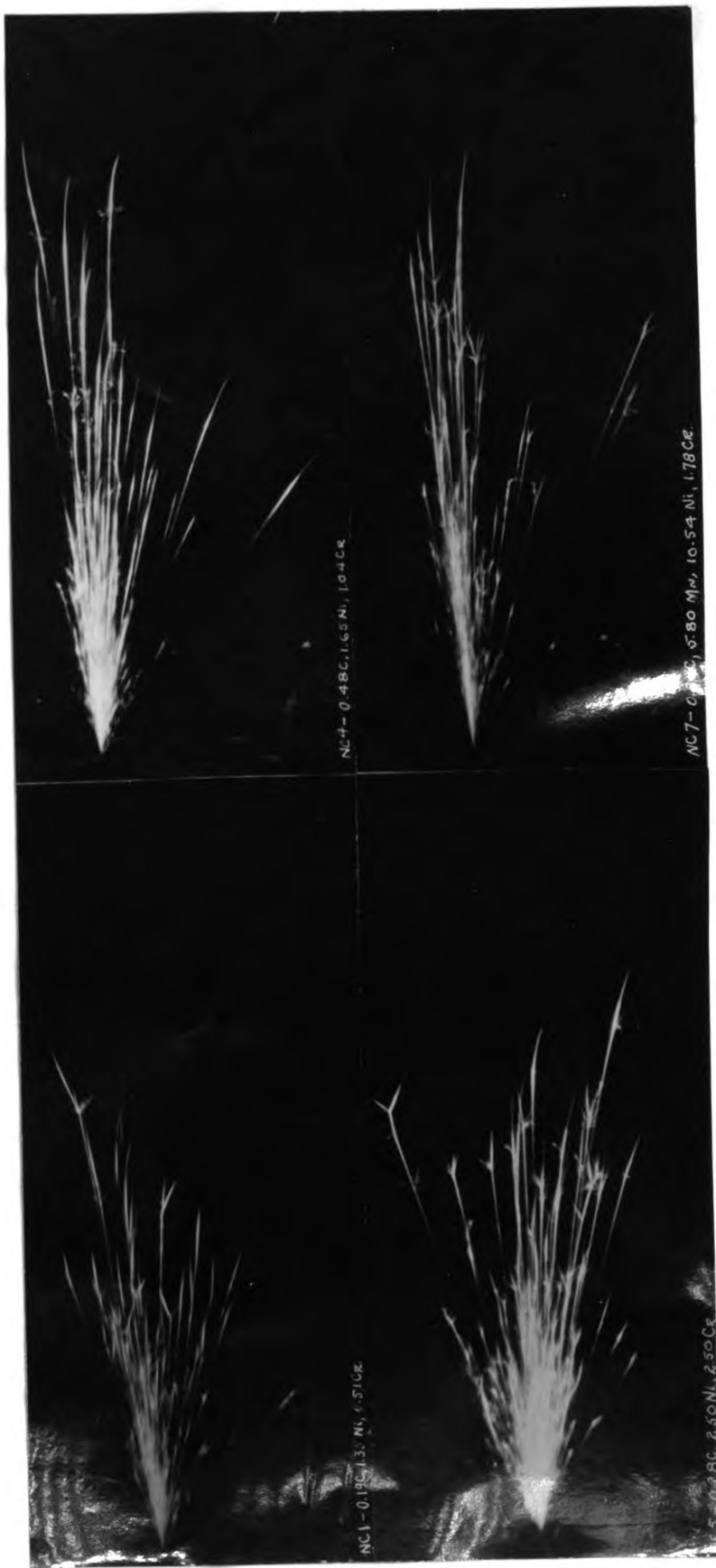
Fig. 11 - Spark streams of special chromium-nickel steels
