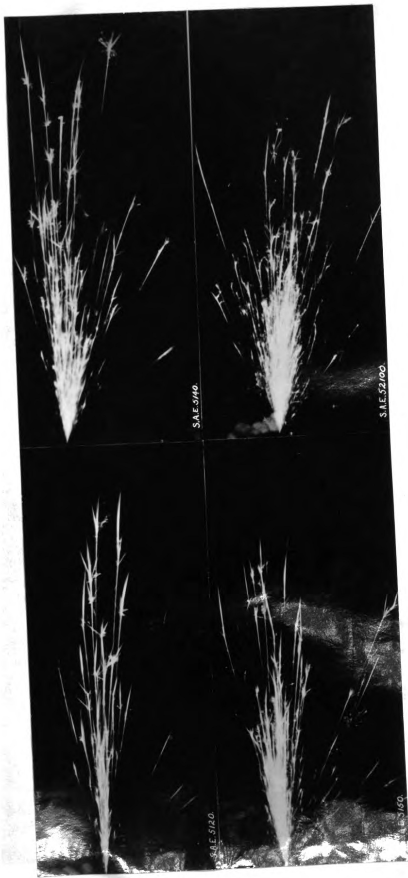
Fig. 6 - Spark streams typical of S.A.E. chromium steels
