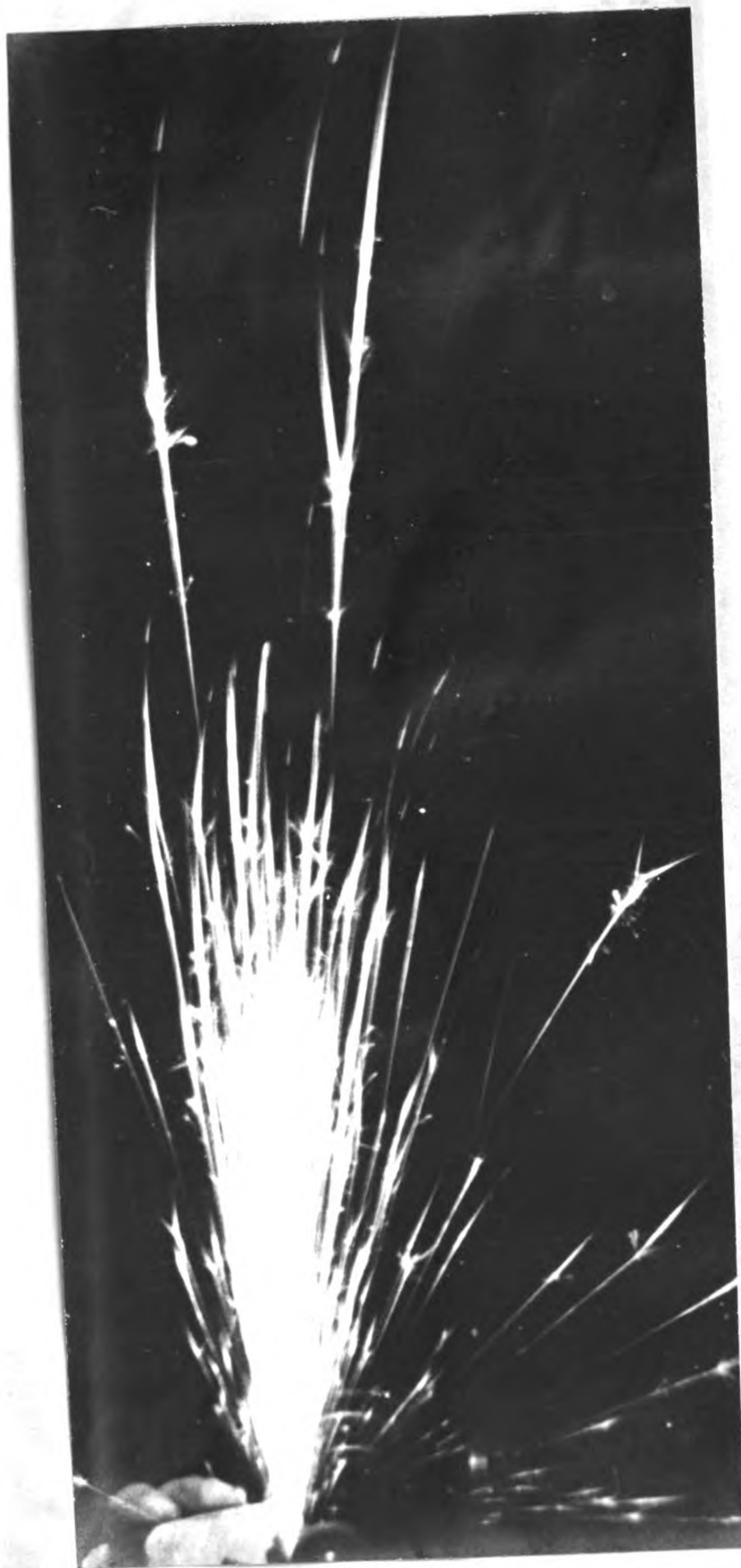
Fig. 14A- Spark streams typical of molybdenum steel showing spearpoints - Type S.A.E. 4130
