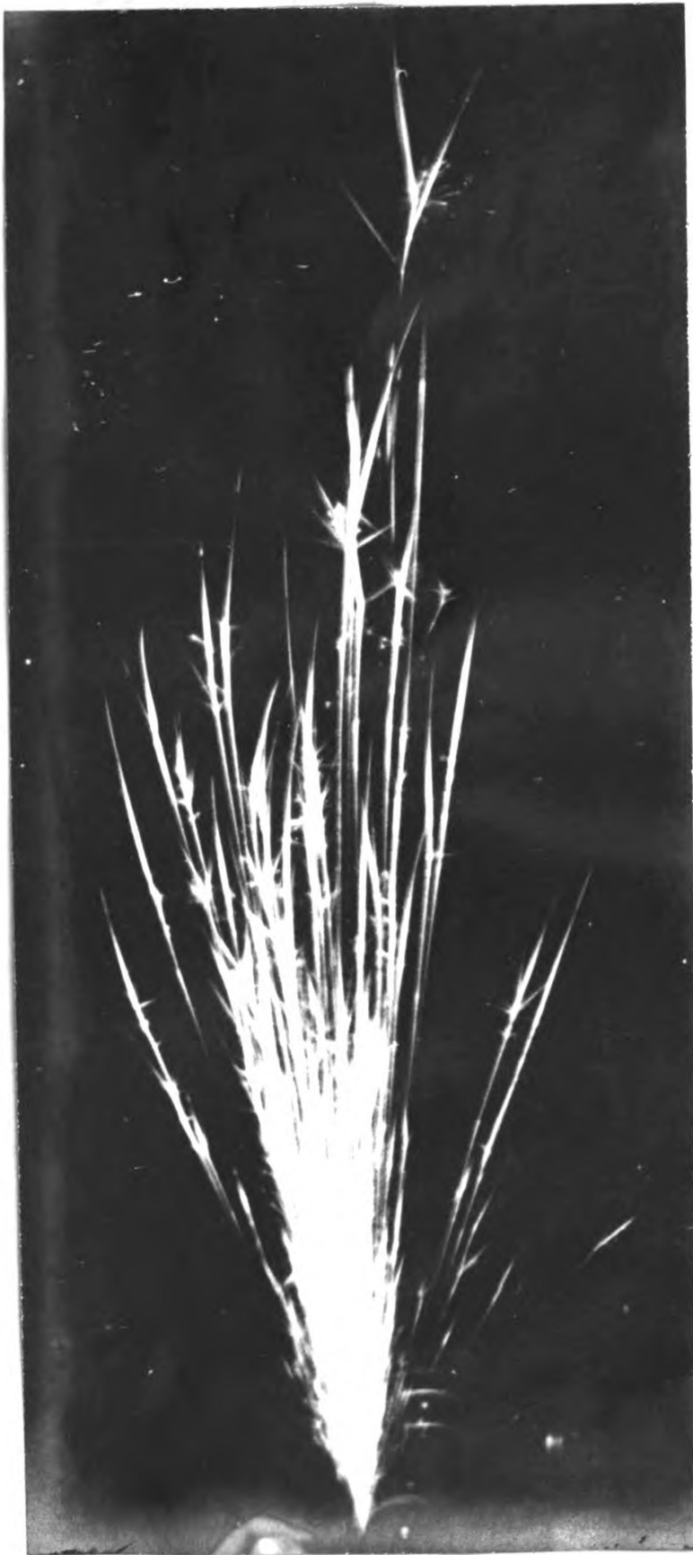
FIG. 4A - Spark streams typical of nickel steels
