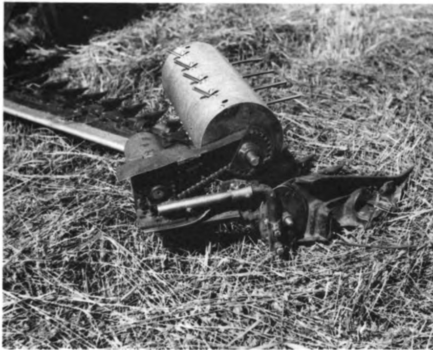
Fig. 6. Powered grass divider assembly.
