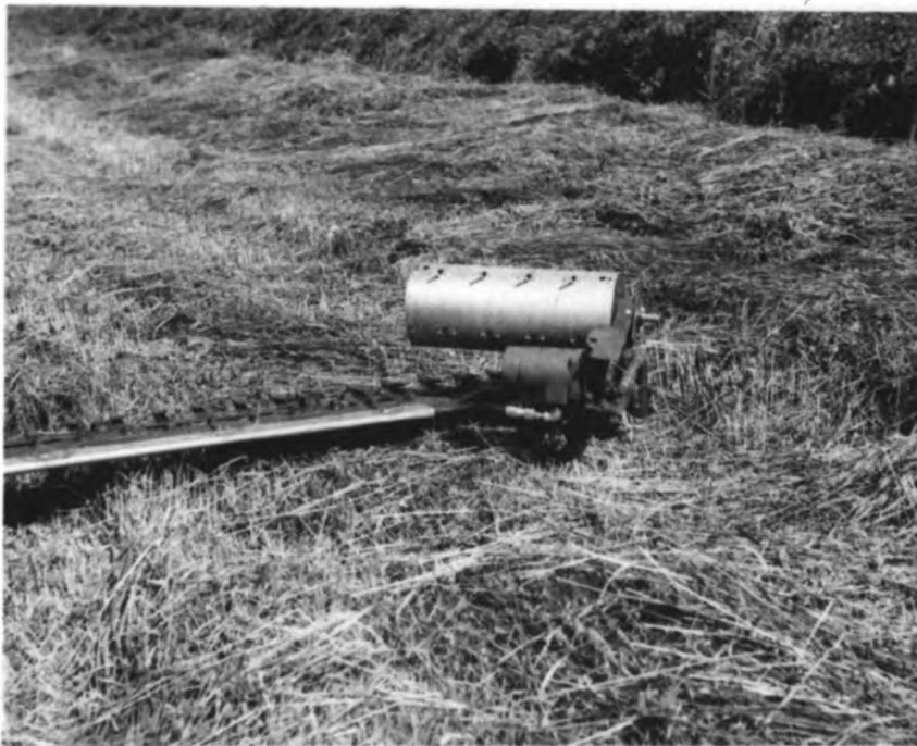
Fig. 7. Mounting position of the hydraulic motor and enclosure of hydraulic lines.
