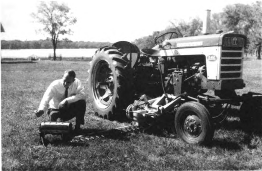
Fig. 2. Tractor and mower with powered grass divider.
