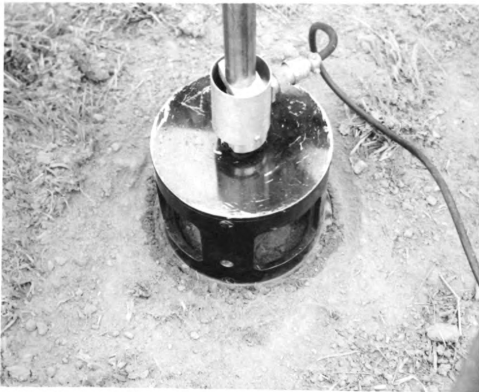
Fig. 22. Shear head in operation.
