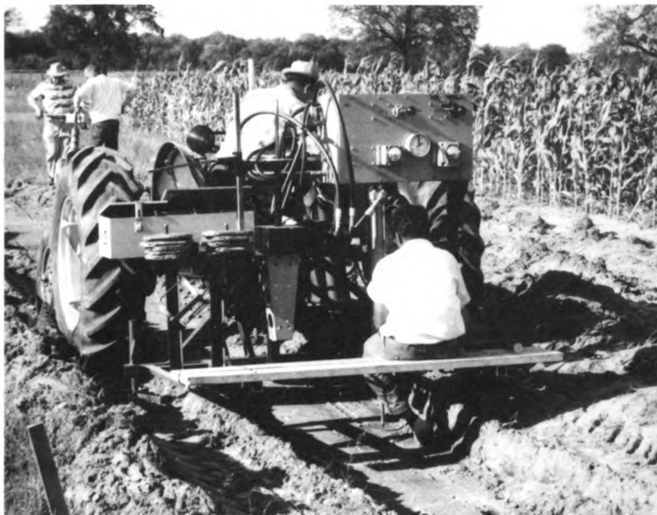
Fig. 10. Bevameter in operation. Operation of powered soil sampler can be seen in the background.
