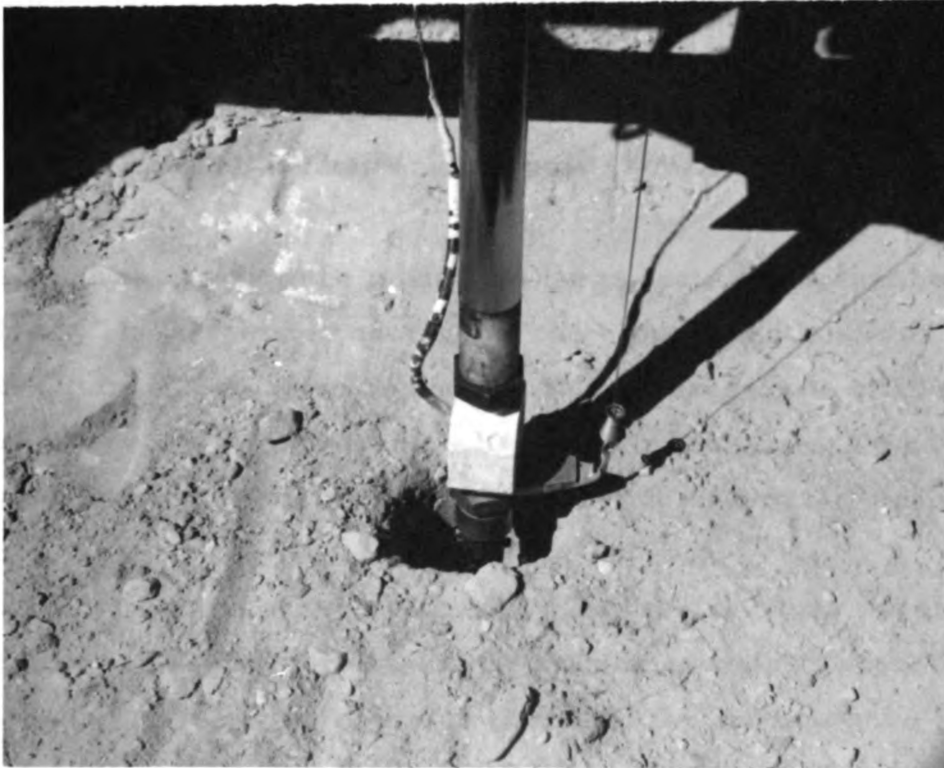
Fig. 20. Penetrometer completely in the soil.
