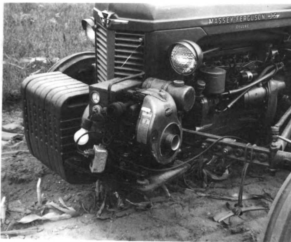
Fig. 16. Electric generator on the tractor front end.
