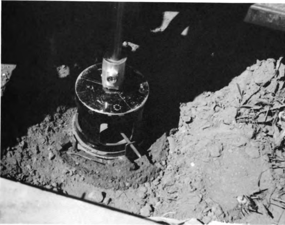
Fig. 21. Shear head with surface planing device attached.
