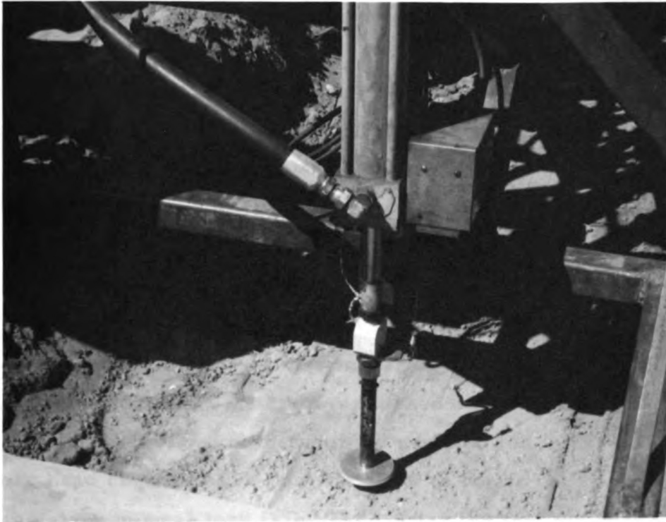
Fig. 19. Penetrometer before forcing into the soil.
