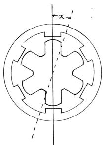
A constant e.m.f. will be induced in the rotor windings, and with a voltmeter it is possible to read the e.m.f. induced.
