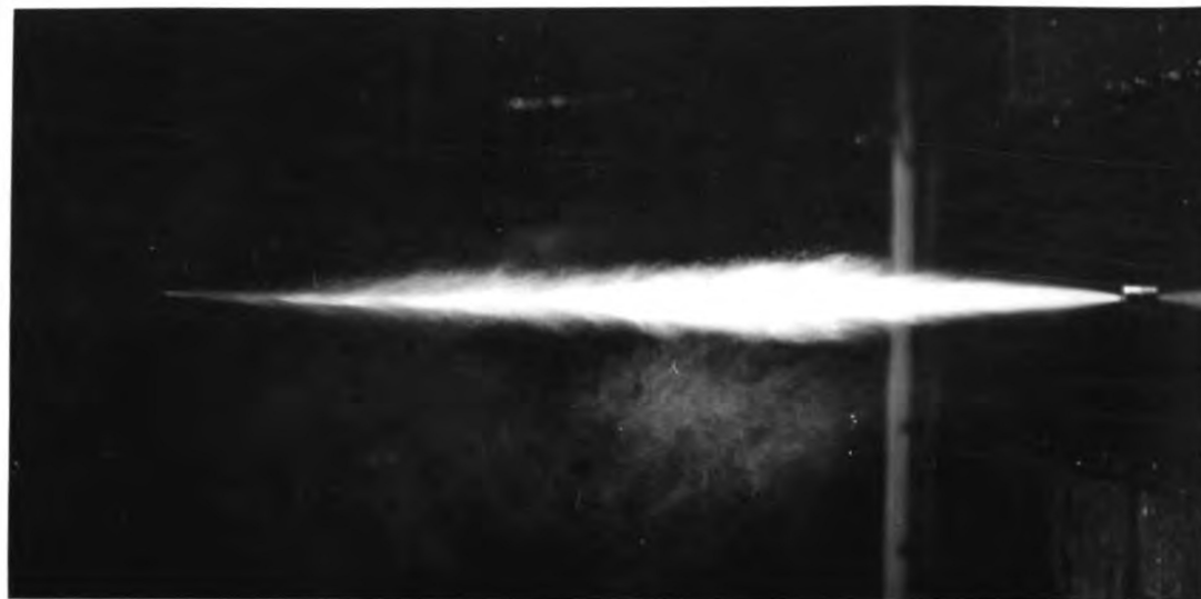
PLATE 9: Injection begins at 5^{\circ} , photo at 19^{\circ} , 250 rpm., .500 inch rack opening, AKC 45 SD 51 narrow pintle nozzle, 11 inch long steel tube, 1000 psi. nozzle opening pressure.
