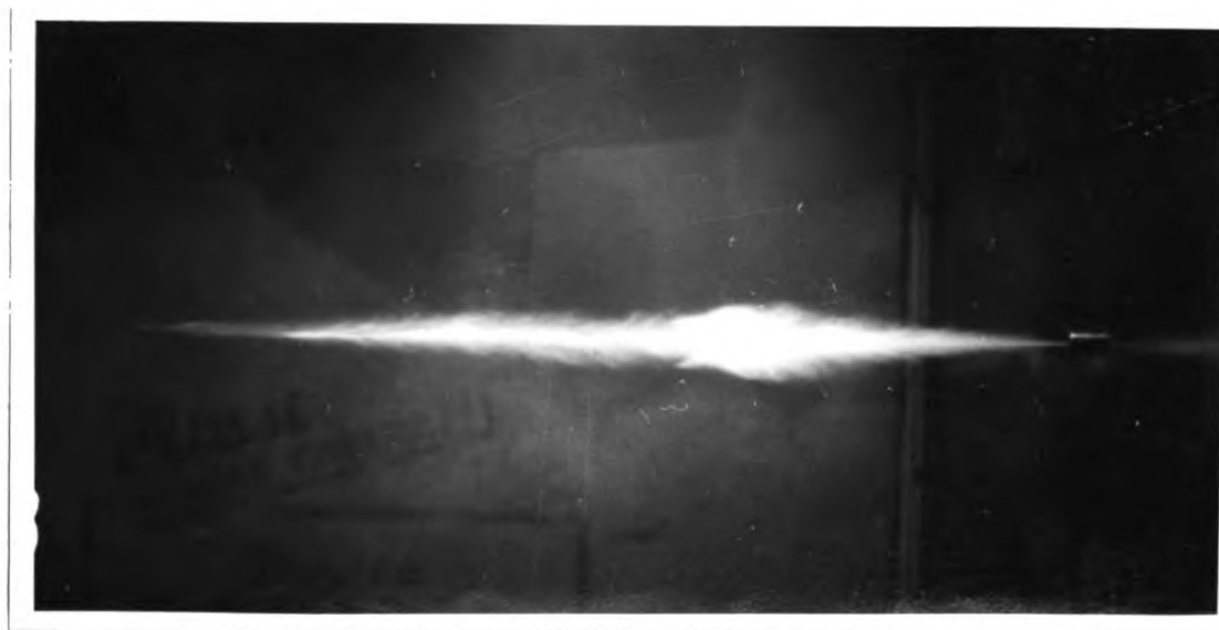
PLATE 8: Injection begins at 4\frac{1}{2}^{\circ} , photo at 15^{\circ} , end of injection at 15^{\circ} , 260 rpm., .375 inch rack opening, AKC 45 SD 51 narrow pintle nozzle, 1675 psi. nozzle opening pressure, 11 inch long steel tube.
