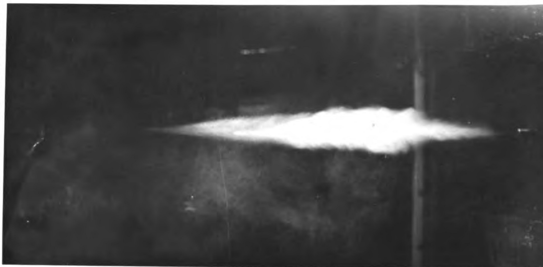
PLATE 19: Injection begins at 3\frac{1}{2}^{\circ} , photo at 16\frac{1}{2}^{\circ} , 250 rpm., .375 inch rack opening, AKB 35 SD 173 medium pintle nozzle, 2000 psi. nozzle opening pressure, 44 inch long steel tube. The end of the first phase.
