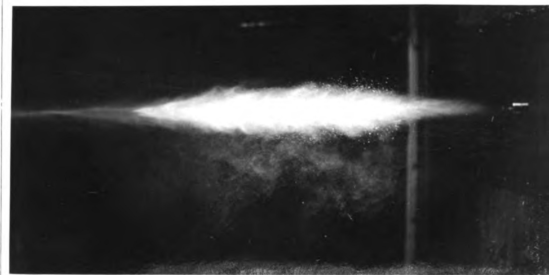
PLATE 13: Injection begins at 5^{\circ} , photo at 17^{\circ} , second phase begins at 16^{\circ} , injection ends at 20^{\circ} , 260 rpm., .375 inch rack opening, AKC 45 SD 51 narrow pintle nozzle, 1675 psi. nozzle opening pressure, 41 inch long copper tube. An illustration of the breakup of the spray near the end of injection.
