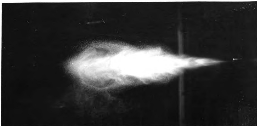
PLATE 23: Injection begins at 9^{\circ} , photo at 18^{\circ} , 250 rpm., .500 inch rack opening, AKB 25 R 75 wide pintle nozzle, 2000 psi. nozzle opening pressure, 44 inch long steel tube. The end of the injection.
