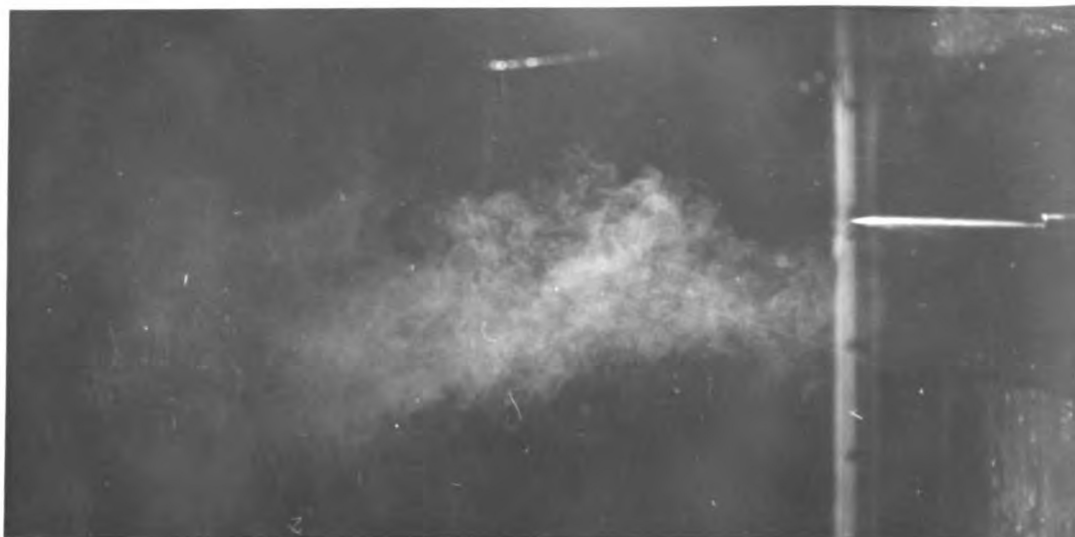
PLATE 17: Injection begins at 3\frac{1}{2}^{\circ} , photo at 7^{\circ} , 250 rpm., .375 inch rack opening, AKB 35 SD 173 medium pintle nozzle, 2000 psi. nozzle opening pressure, 44 inch long steel tube. The first stage of injection of this nozzle.
