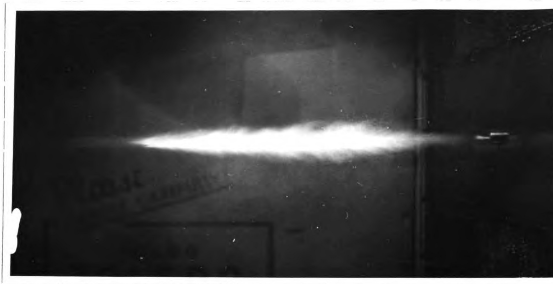
PLATE 13: Injection begins at 5^{\circ} , photo at 17^{\circ} , second phase begins at 16^{\circ} , injection ends at 20^{\circ} , 260 rpm., .375 inch rack opening, AKC 45 SD 51 narrow pintle nozzle, 1675 psi. nozzle opening pressure, 41 inch long copper tube. An illustration of the breakup of the spray near the end of injection.
