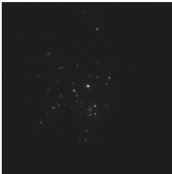
Figure 1.1. Wide-field image of a silver nanoparticle film collected without scanning either the laser or the sample. The entire image is 80 \times 80 \mu\text{m} , and the laser was focused near the center. Rather than observing bright emission at the focus against a black background, discrete regions of luminescence remote from the focal spot are observed, indicating that some mechanism for energy transport exists in the nanoparticle network.
