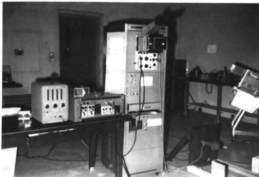
Instrumentation. Counter and relay for switches. Amplifiers, oscilloscope and POLAROID camera. Backstop of test track and light beam trigger.
