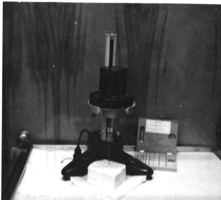
Fig. 9. Brookfield viscometer positioned for viscosity measurements on butter.
