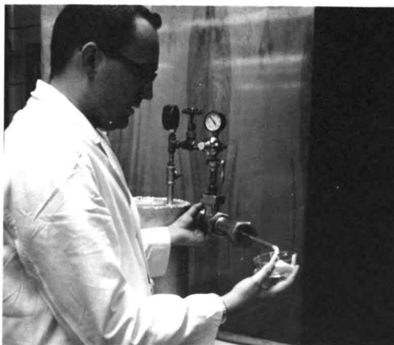
Fig. 7. Extrusion viscometer in operation.
