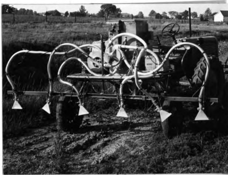
Figure 13. The field duster X1 prior to modification from a six outlet to an eight outlet machine.
