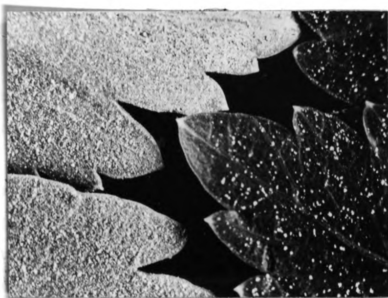
Figure 5. Upper surface of dusted celery leaves magnified approximately five times. Leaf on the left charged dust; leaf on the right uncharged dust.
