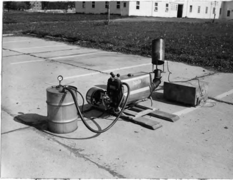
Figure 20. Dyna-Fog fog generator. Box on the right contains the electrical power supply. The charging nozzle is attached to the fog outlet.
