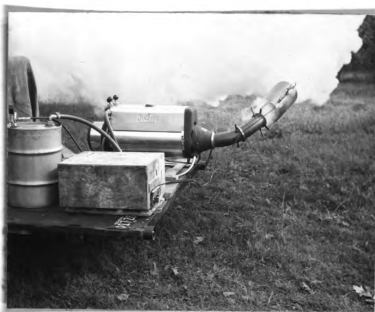
Figure 23. Dyna-Fog fog generator in operation. Drum on left contains fog oil.
