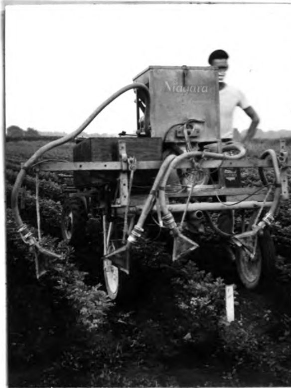
Figure 18. Rear view of the Niagara Cropmaster duster adapted for electrostatic dusting. The box on the left of the machine, just in front of the main beam, contains all the electrical equipment.
