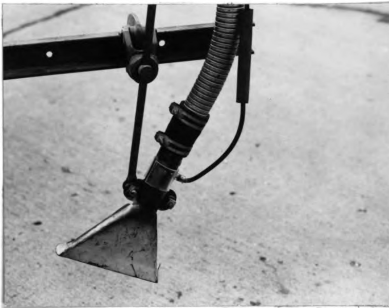
Figure 17. Duster X1, outlet nozzle of one of the tubes showing how the type V charging nozzle is attached.
