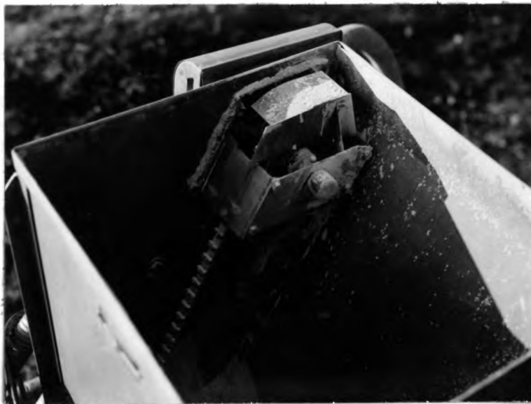
Figure 14. View inside the dust hopper of duster X1 showing the small V-belt conveyor which maintains a constant level in the small upper hopper.
