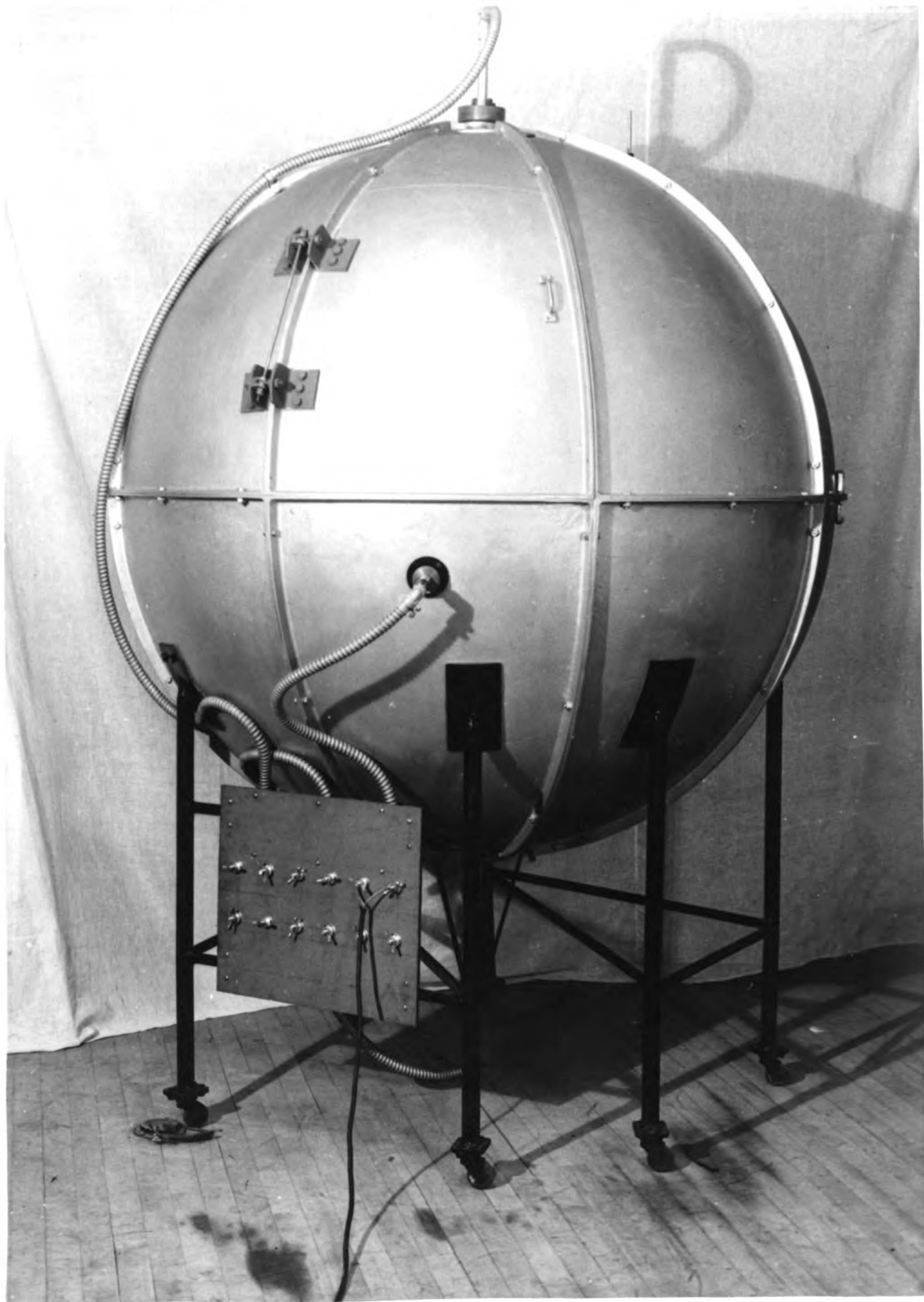
ASSEMBLED SPHERE WITH CLOSE VIEW OF SUPPORTING STRUCTURE AND TERMINAL PANEL FOR CURRENT AND POTENTIAL LEADS
