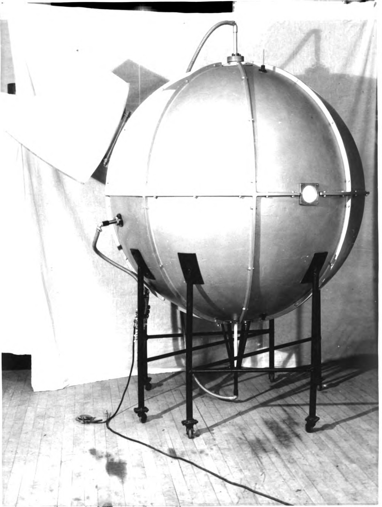
SPHERE PHOTOMETER WITH DOOR OPEN WINDOW TO THE RIGHT
