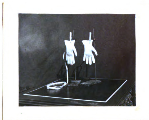
Showing method of securing circumference measurements. The glove on the left is the original, the one on the right has been worn one year.
