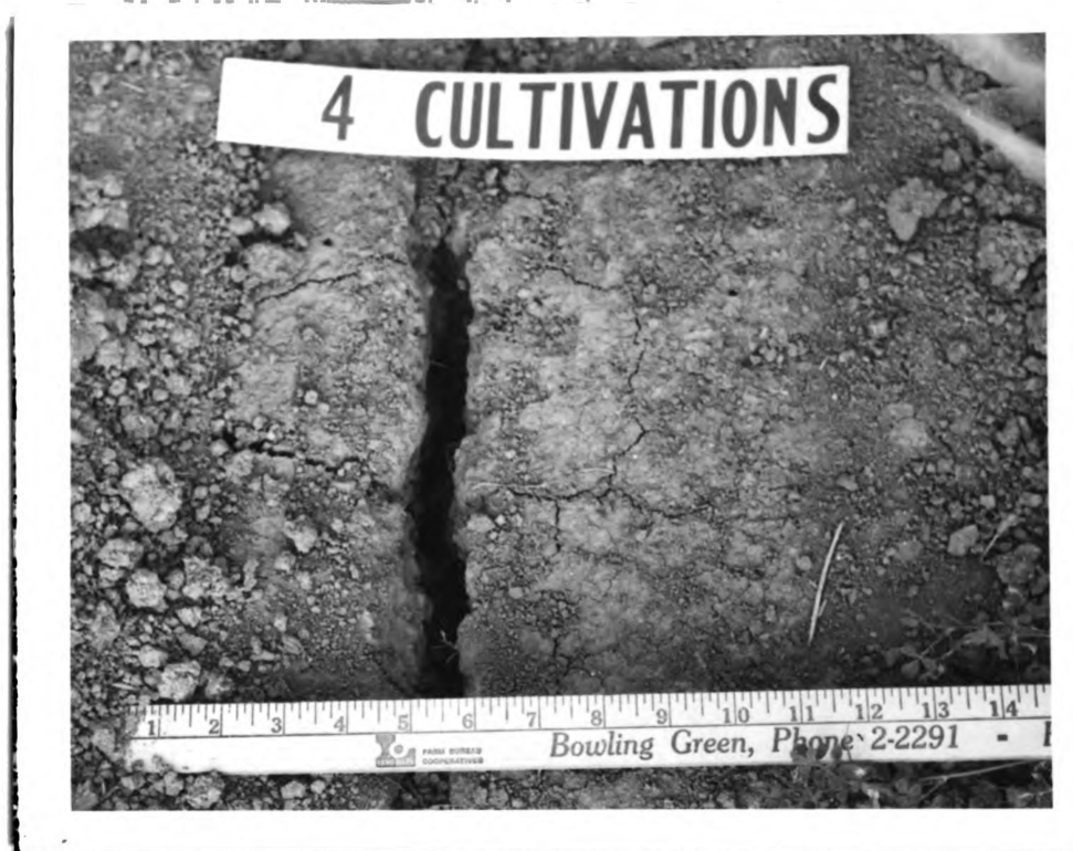
Figure 2. An average of 82.4 blows were required to obtain a core in this area over which the rear wheel of tractor had passed four times during the cultivation.
