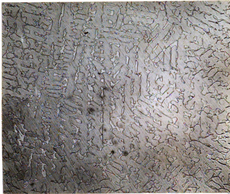
Figure 9. Microstructure of a cast 2.26% Be-97.58% Cu alloy after solution heat treatment at 1470°F. for 15 minutes. Magnification: 100X Etchant: \text{FeCl}_3
