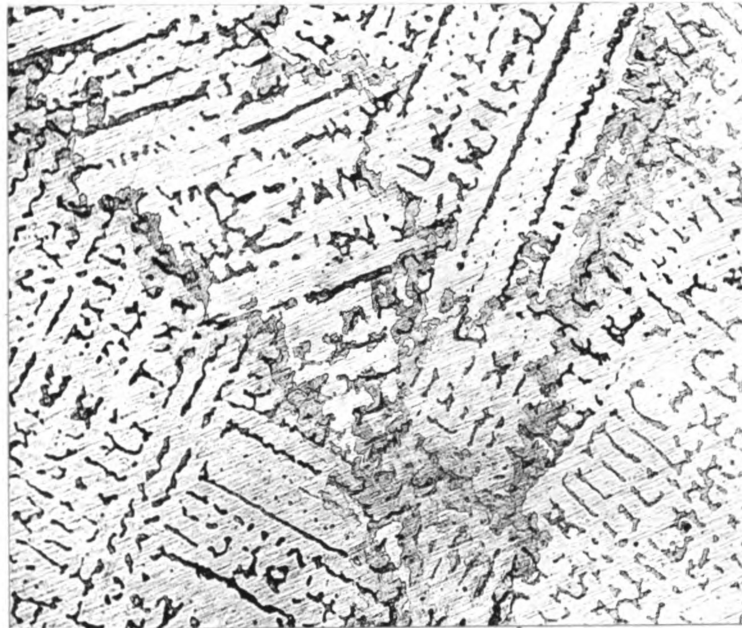
Figure 4. Microstructure of a 2.26% Be-97.58% Cu alloy in the "as cast" condition. Magnification: 100X Etchant: \text{FeCl}_3
