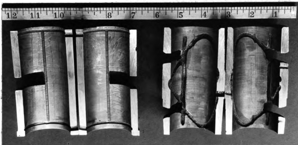
Fig. 16. Lft.-Narrow Sharp Edged Dist. Groove Running Into Drain Grooves. Rt.- Bad Pear Shaped Groove Connecting High and Low Pressure Areas. Bronze Bearings.
