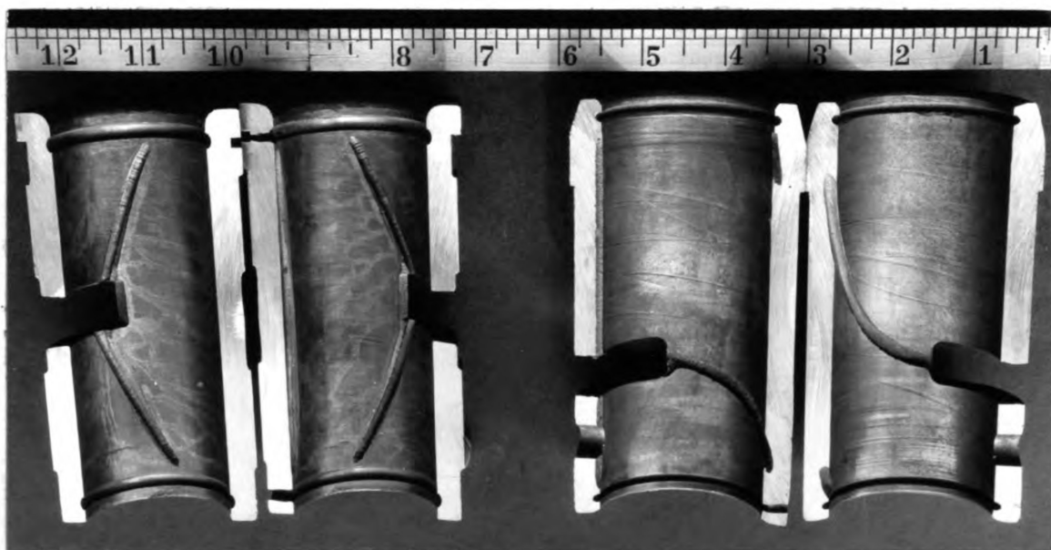
Fig. 17. Lft.- Slanting Grooves Run Into Ring Groove Too High. Rt. - Grooves Connect High and Low Pressure Areas. One Adds Oil While Other Robs.
