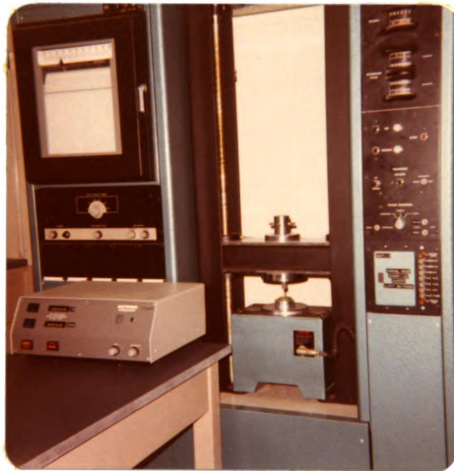
FIGURE 2 PHOTOGRAPH OF THE INSTRON MACHINE AND AREA INTEGRATOR USED FOR CARPEL STRENGTH TESTS.
