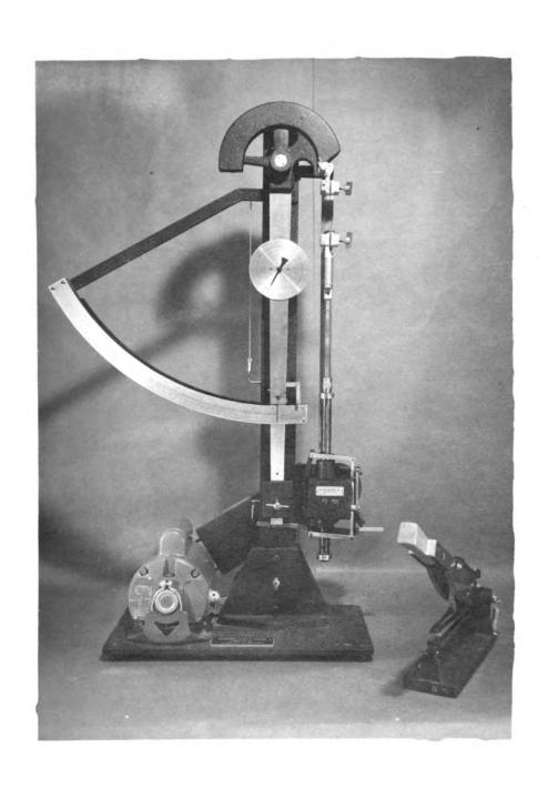
defined as the breaking load divided by the original width of the test specimen (2). Because of the design of the testing machine, the breaking factor is based on the maximum strength which is not necessarily the strength at break.
