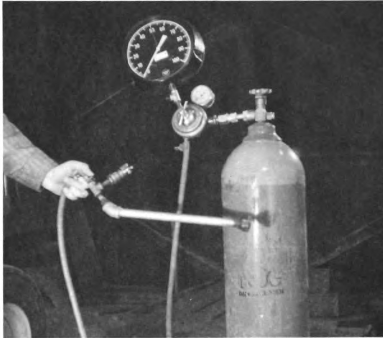
Fig. 8 In Place Calibrator For CST-1 Cells
