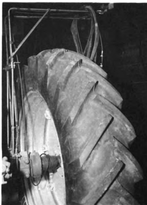
Fig. 18 View Of Gages And Lead Wires From Tractor
