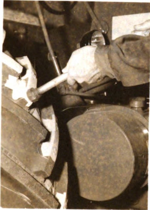
Fig. 10 Pressure Applicator In Place On A Cell
