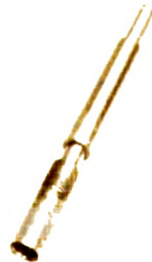
Fig. 13 Drill For Cutting Cell Holes In Tire
