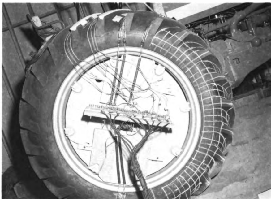
Fig. 19 Side View Of Wheel Showing Lead Wires
