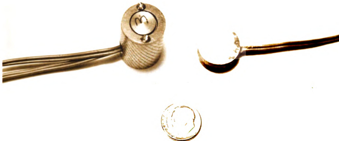
Fig. 2a Picture Of Assembled CST-1 And Diaphragm Cell
