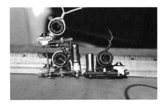
Figure 4. Transmitter, oscillator section.
