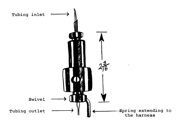
Figure II. Swivel mechanism.
