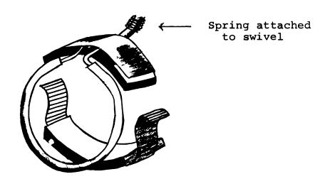
Figure III. Harness for holding the rat.
