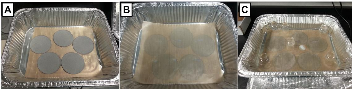
Figure 2.14: Leeching process to remove PEI consisting of (A) placing dried GNP/PP papers onto a porous PTFE cloth (B) covering with a second porous PTFE cloth and (C) filling with water and stirring at room temperature for over 12 hours
