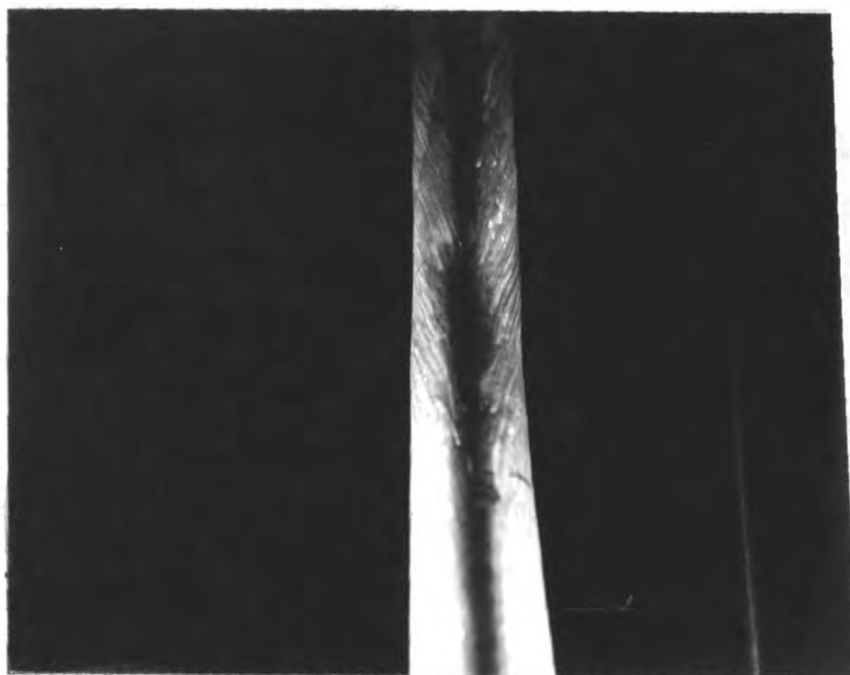
Fig. 31 Bottom view of secondary flow in the boundary near the tube wall at the bend.
