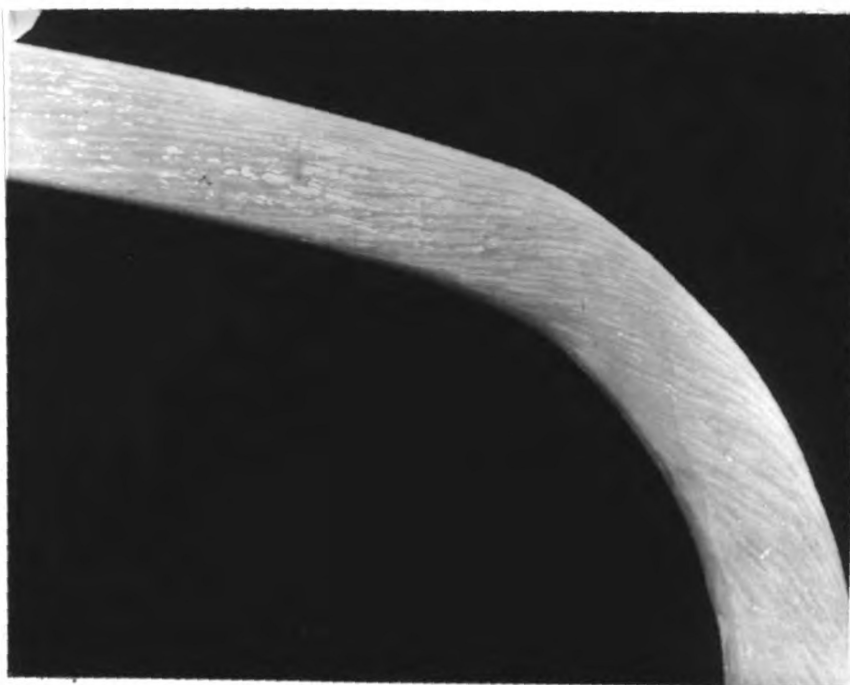
Fig. 29. Side view of secondary flows in the boundary near the tube wall at the bend.
