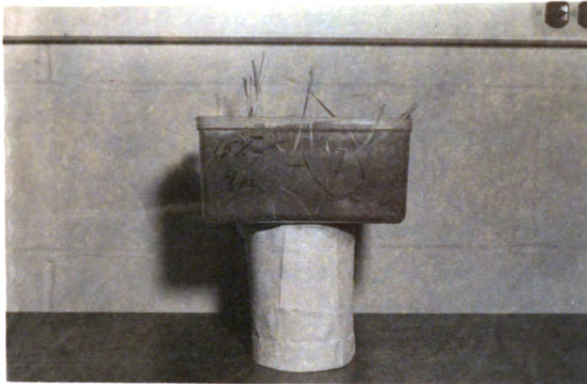
Figure 13: Seedlings Growing Horizontally to Emerge From Loose Soil Near the Wall of the Box. Initial Moisture Content 15%, Compaction 8 psi
