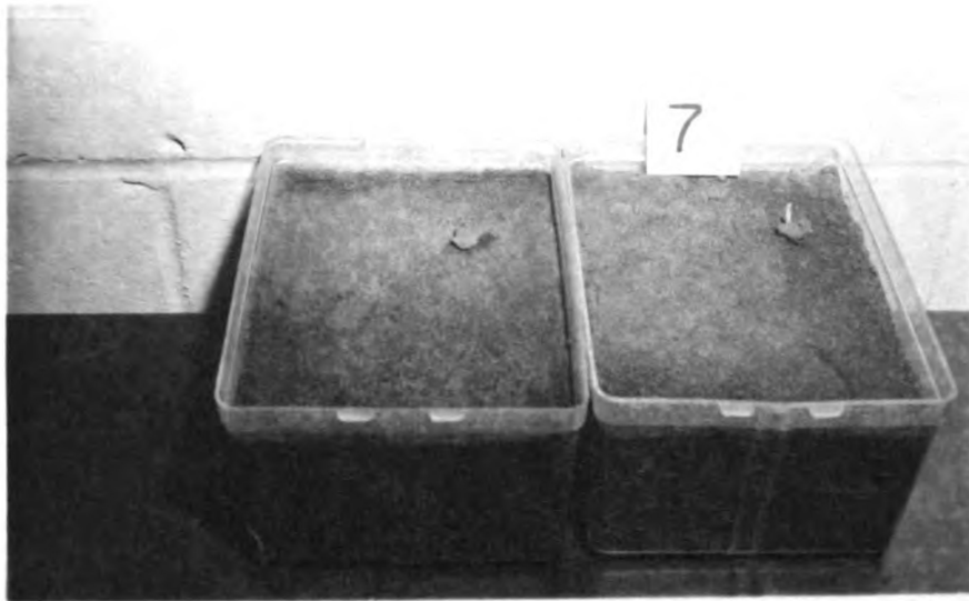
Figure 18: The Similarity Between the Soil Cone Produced by the Mechanical Seedling (at left) and the Cone Produced by Plant Seedling (at right)
