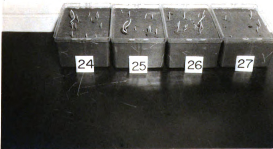
Figure 24: The Effect of Soil Moisture Content on Emergence. The Three Treatments Had Almost Identical Emergence Force (about 0.60 pounds)
