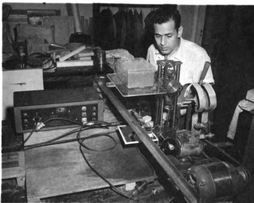
Figure 2: View of the Penetrometer System Showing the Rigid Support for the Simply Supported Beam
