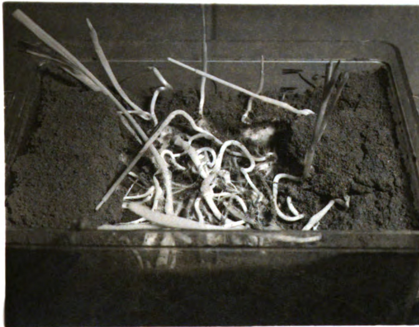
Figure 14: Top View of a Sample With Initial Moisture Content 15% and Compaction Pressure 8 psi After Lifting a Block of Soil that Weighed 450 Grams. Seedlings Are Buckled Severely
