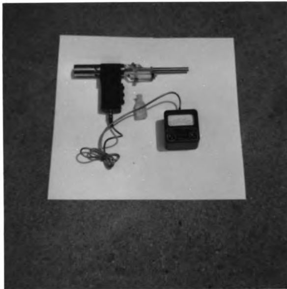
Figure 9. "Hygrophil" thermistor psychrometer, with indicating meter and distilled water reservoir.
