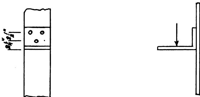
Test for tension in top rivets.
