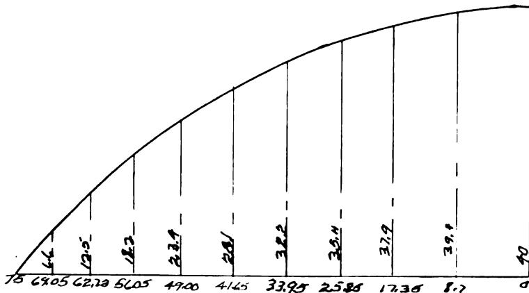
Bending moment at any section is equal to the summation of moments to either side of the section.
