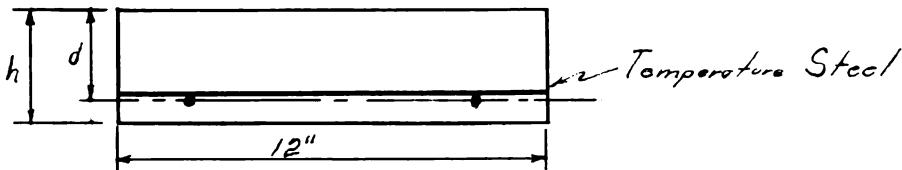
Cross section through slab unit.
